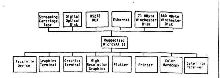
Figure 2. Block diagram of the Weather-Intensive ATS Processor.
