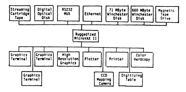
Figure 3. Block diagram of the Terrain-Intensive ATS Processor.
