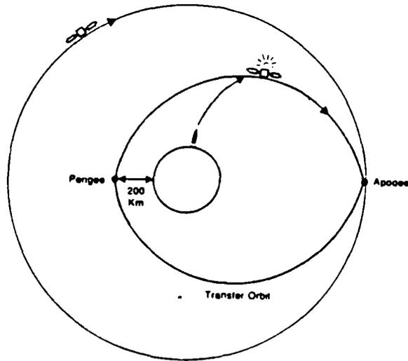
Figure 2.2 (a.) Launch Geometry - Expendable Vehicle
