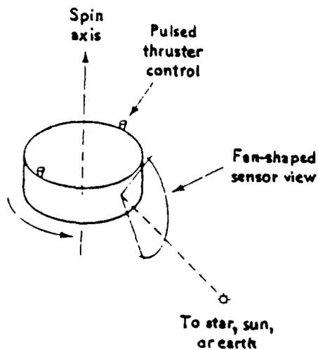
Figure 2.1 Spin-stabilization [Ref. 2: p. 115]
