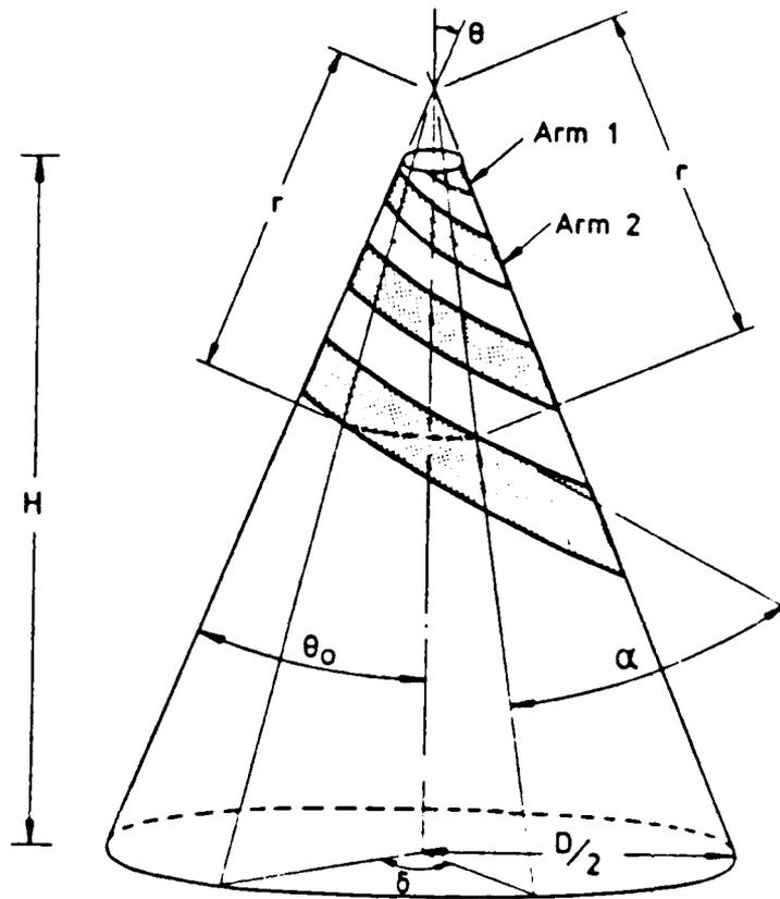
Figure 3.12 Conical Log-Spiral Geometry
