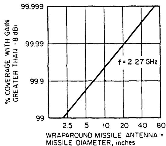
Figure 3.8 Coverage Versus Diameter
