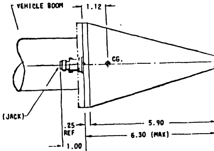
Figure 3.15 Antenna Dimensions
