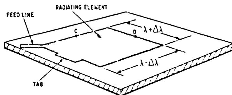
Figure 3.6 Circularly Polarized Element
