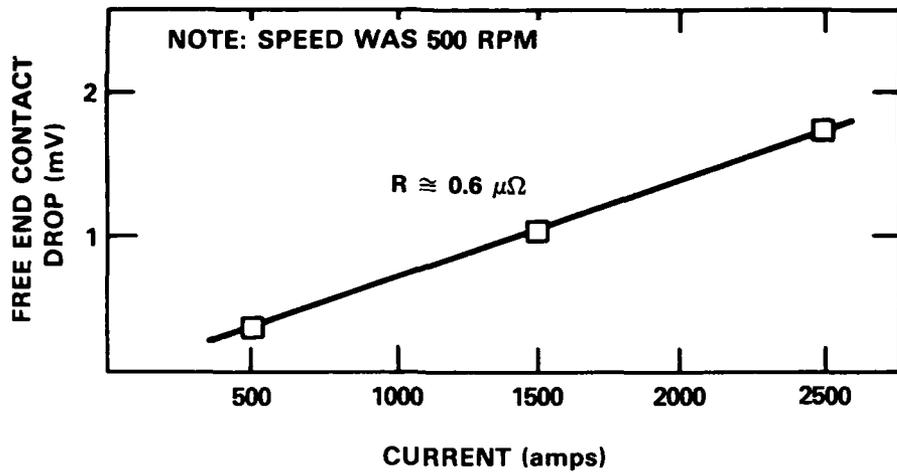
Fig. 5. Effect of current on contact drop.
