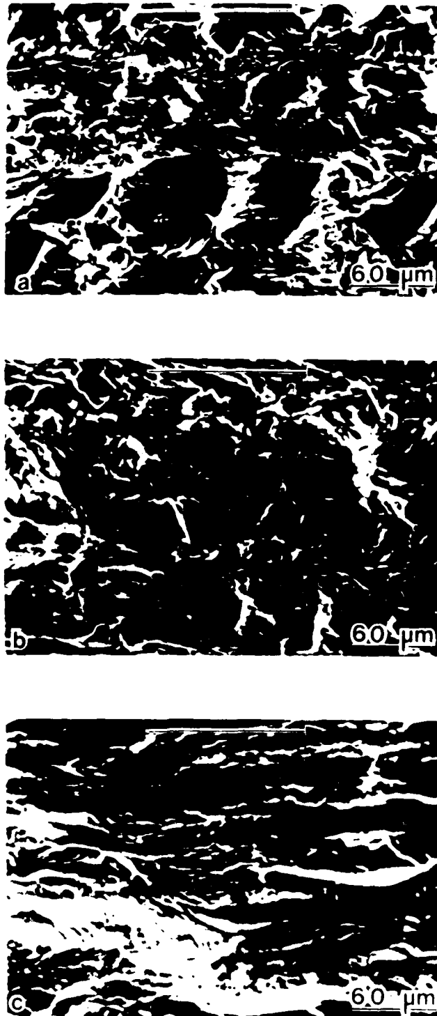
Fig. 4.4: Scanning electron micrographs of fatigue fracture surfaces close to \Delta K_{TH} ( R = 0.10 ) in I/M 7150 aluminum alloy, showing the morphology in a) underaged, b) peak-aged (T6) and c) overaged (T7) microstructures.
