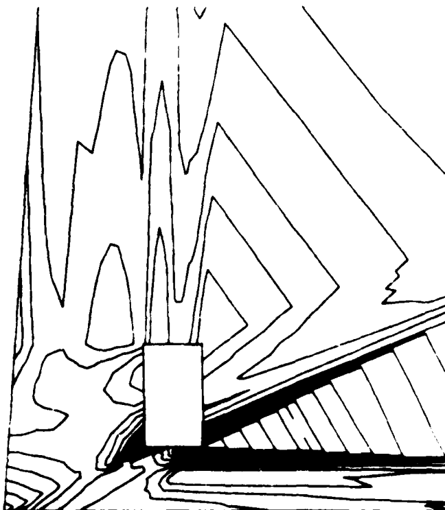
Figure A35. Subwindow plot of nonannotated, Y-direction principal stress contours, coarse grid, P-level 6
