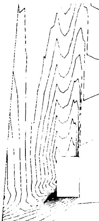
Figure A11. Window plot of nonannotated, Y-direction stress contours, coarse grid, P-level 1
