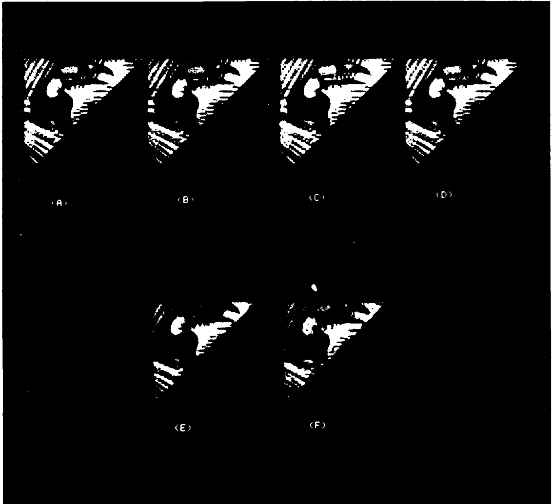
Figure 3. Examples of reconstructing objects from the moduli of their transforms using a triangular support constraint. (a) Object with sharp edges and bright corners, (b) reconstructed image; (c) object with sharp edges and zeroed corners, (d) reconstructed image; (e) object with tapered edges and zeroed corners, (f) partially reconstructed image.
