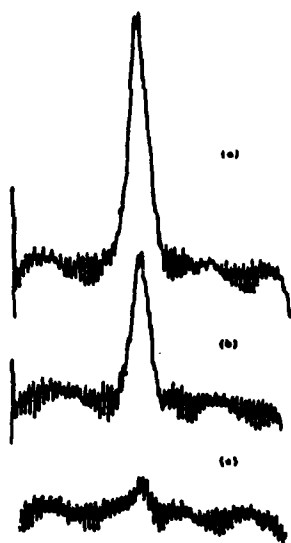
Fig. 4. Cross-correlation signals due to a MSF of a 10-line ruling pattern on the LCTV screen addressed by (a) 10 lines, (b) 24 lines, (c) a blank screen. The vertical axes are of the same scale with arbitrary units. The horizontal axis has a total width of 3.2 mm ( =128 \mu\text{m} \times 25 \mu\text{m} ).
