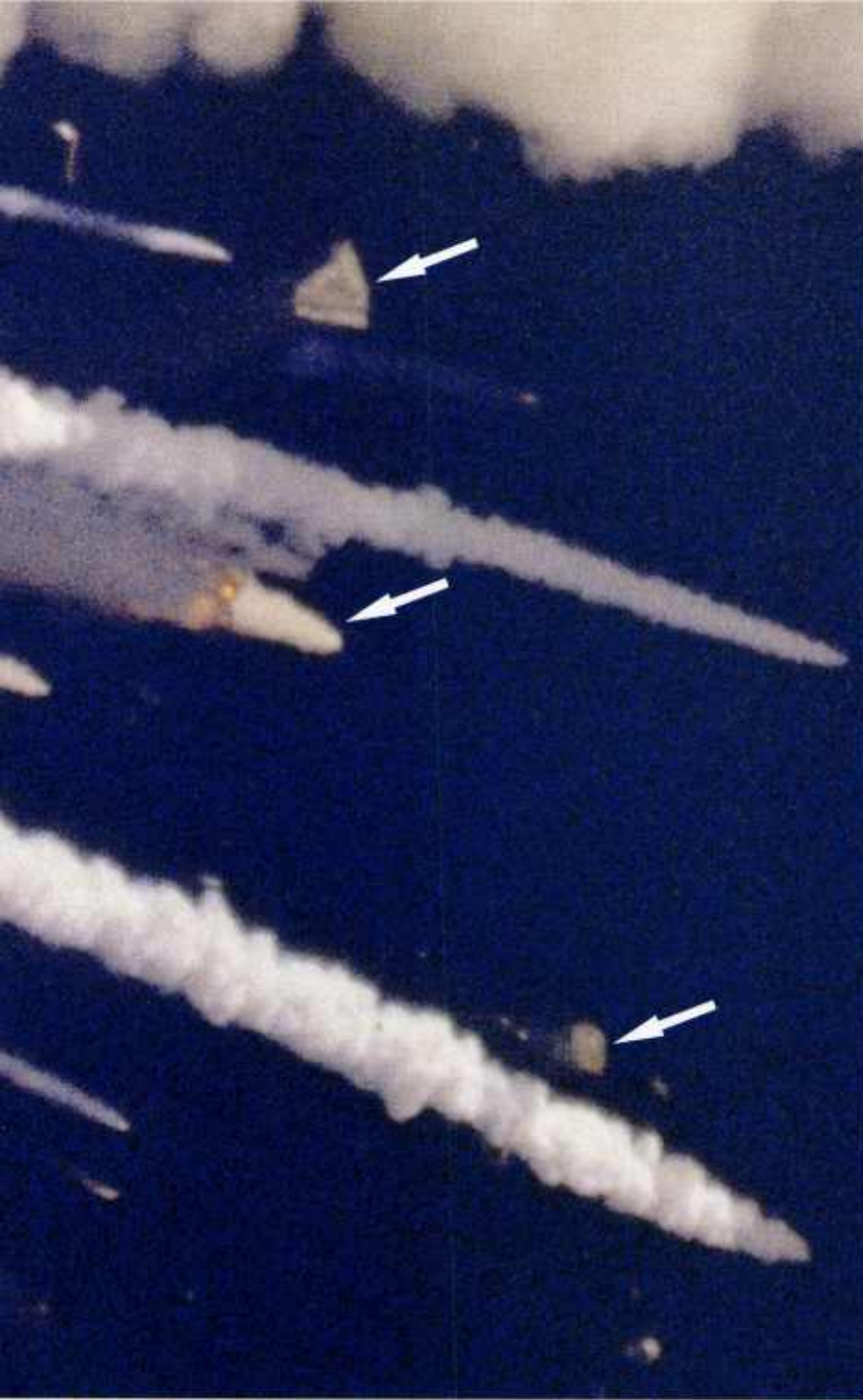
Hurling out of the fireball at 78 seconds (left) are the Orbiter's left wing (top arrow), the main engines (center arrow) and the forward fuselage (bottom arrow). In the photo below, it plunges Earthward, trailed by smoking fragments of Challenger.
