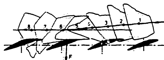
Successive stages of ice impact to propeller blade.
