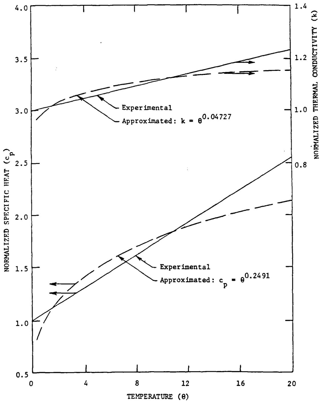
Figure 3. Thermal Properties of Type 420 Stainless Steel (normalized)
