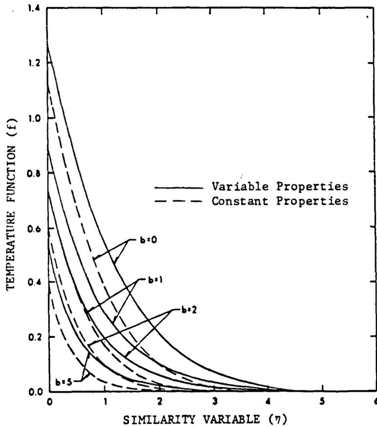
Figure 4. Profiles of Temperature Function (boundary condition  $Q_w = at^b$ )
