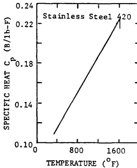
Figure 1. Thermal Properties of Type 4130 Steel and Type 420 Stainless Steel (reproduced from Ref. 2)
