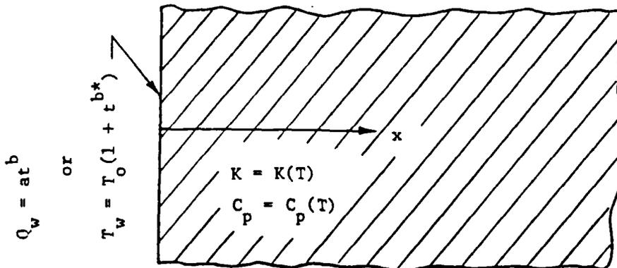
Figure 2. Semi-infinite Solid with Temperature-Dependent Thermal Properties
