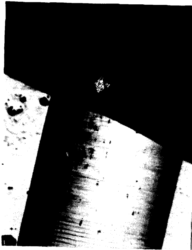
Figure 5. Nomarsky photomicrograph of a typical cut at the point of entry into the specimen.
