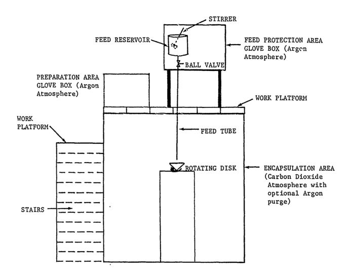
Figure 3. Side View of Enclosure Built to Provide an Inert Atmosphere for Encapsulation of Lithium Metal.
