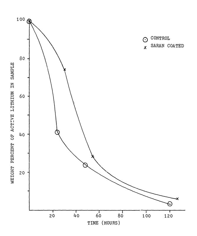
Figure 5. Effects of Saran Coating on Run 2-1 Reported as Active/Payload\*100% at 23°C and 50% K.H.
