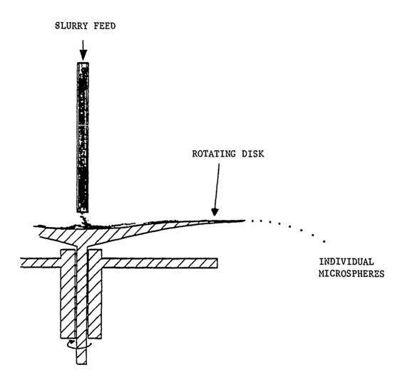
Figure 2. Schematic View of Formation of Microspheres From the Rotating Disk.
