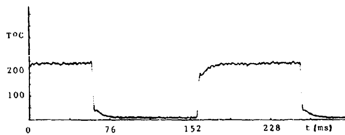
Fig. 10 Compensated junction temperature history (laser heating)
