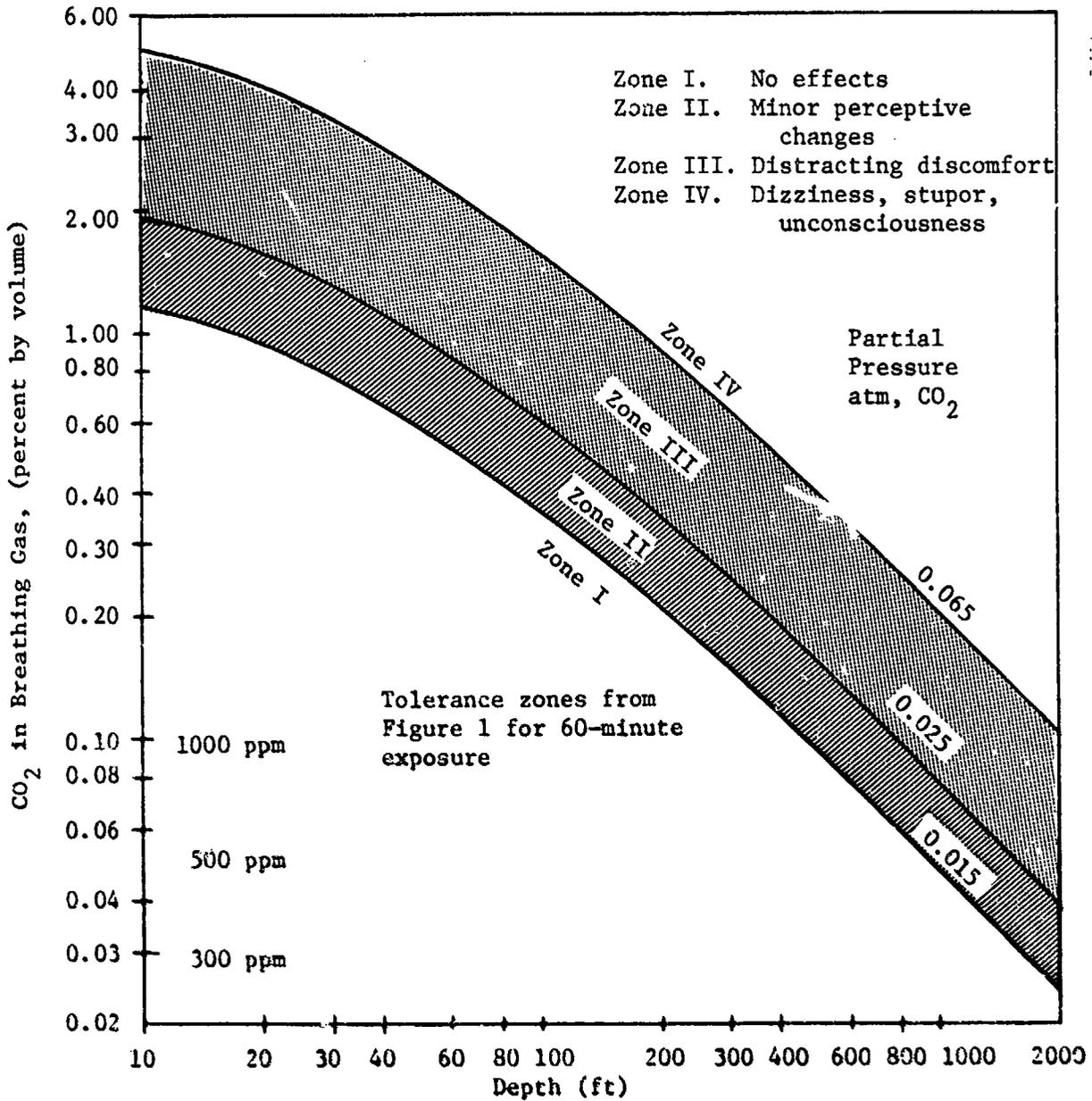
FIGURE 2. RELATION OF CO<sub>2</sub> TOLERANCE ZONES TO DEPTH AND PERCENTAGE OF CO<sub>2</sub> IN BREATHING GAS
