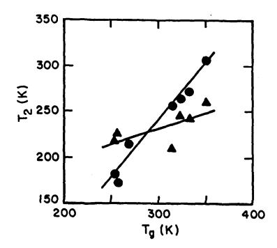
8. Gibbs-DiMarzio second order transition temperature,  $T_2$ , versus glass transition temperature of DGEBA. triangles -  $\sigma_{\rm c}$  circles -  $f_{max}$
