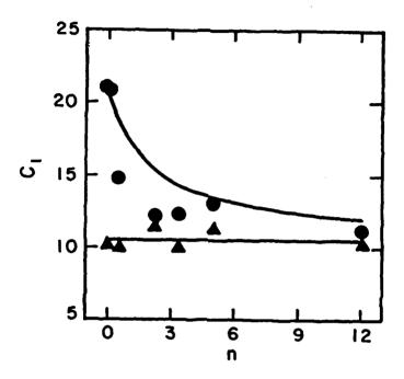
7. WLF constant  $C_1$  versus mer index n of DGEBA. triangles -  $\sigma$ , circles -  $f_{max}$
