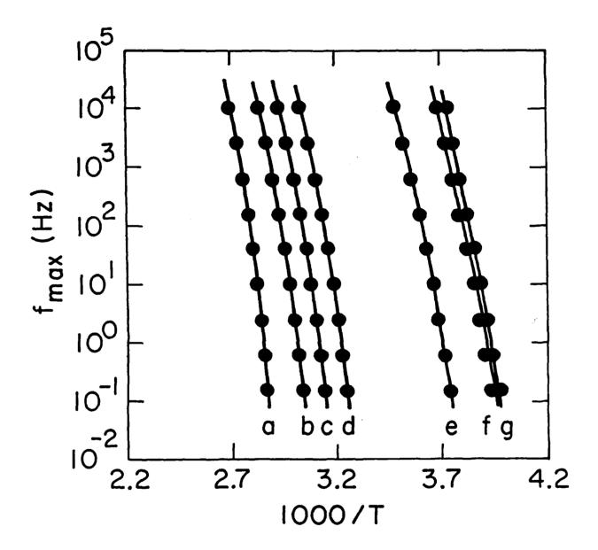
Arrhenius plot of frequency of maximum dipole loss, f<sub>max</sub>, of EPON resins.
