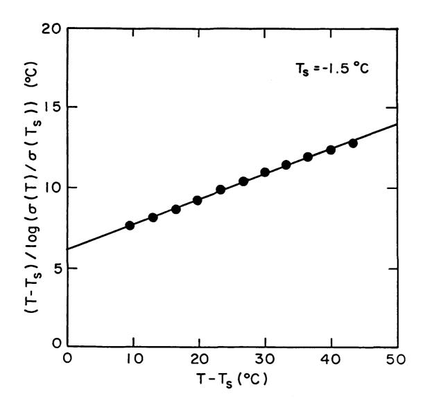
6. Test plot of Williams-Landel-Ferry equation for EPON 828 ionic conductivity data, using a reference temperature of -1.5°C.
