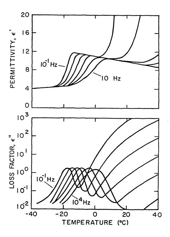
Permittivity, s', and loss factor, s", versus temperature for EPON 828 at frequencies of 0.1, 1, 10, 100, 1000 and 10,000 Hz.
