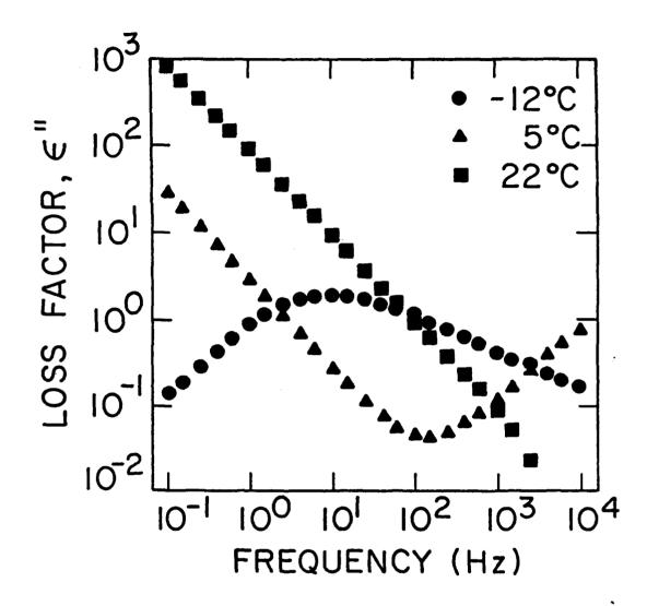
3. Loss factor, s", versus frequency for EPON 828 at temperatures of -12°C, 5°C and 22°C.
