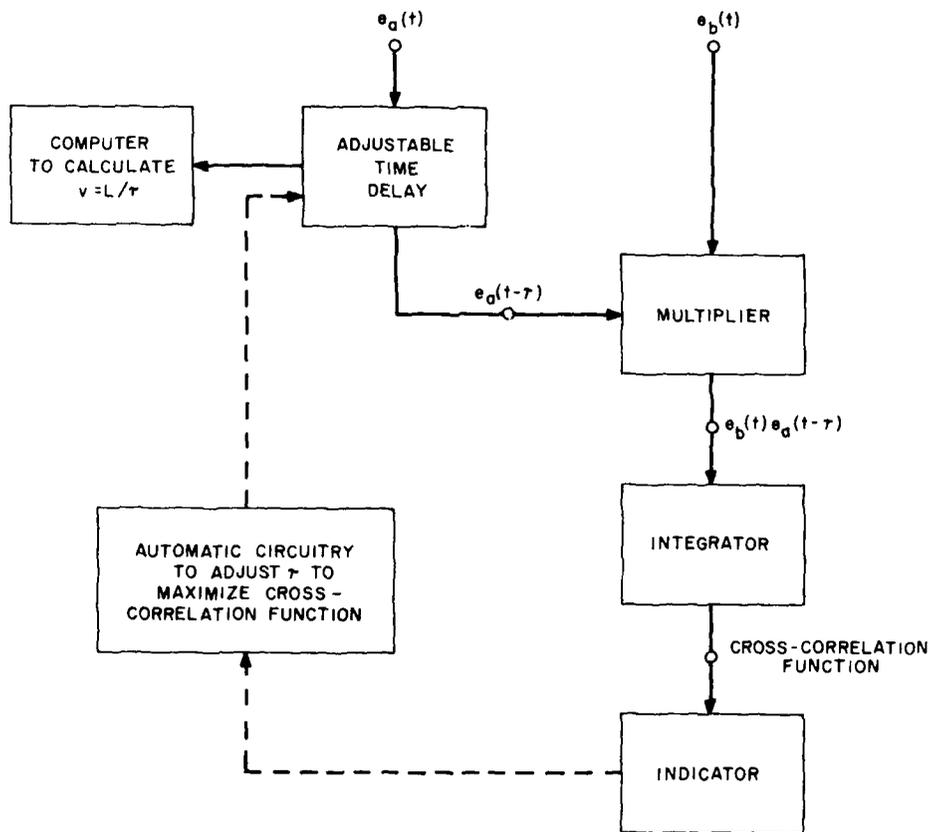
Figure 8. Simple Cross-Correlation Circuitry for Measuring Speed
