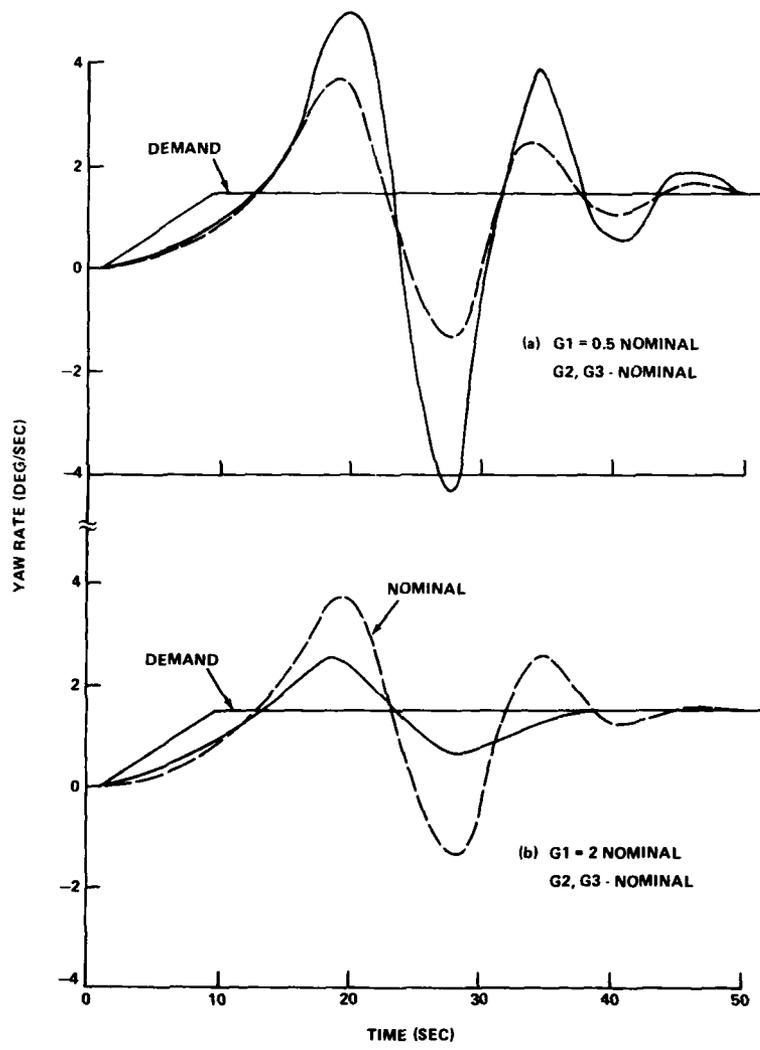
FIGURE 8. SENSITIVITY OF TURN RATE WITH RESPECT TO VARIATIONS IN G1 AT 50 kt
