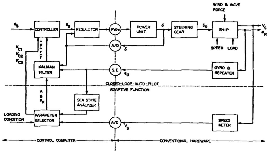
Fig. 2 Block Diagram of New Auto Pilot System
