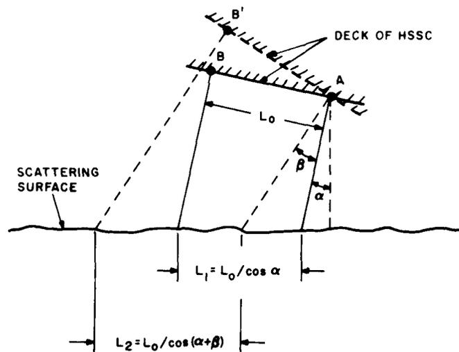
Figure 9. Beam Geometry for Cross-Correlation Speed Sensor
