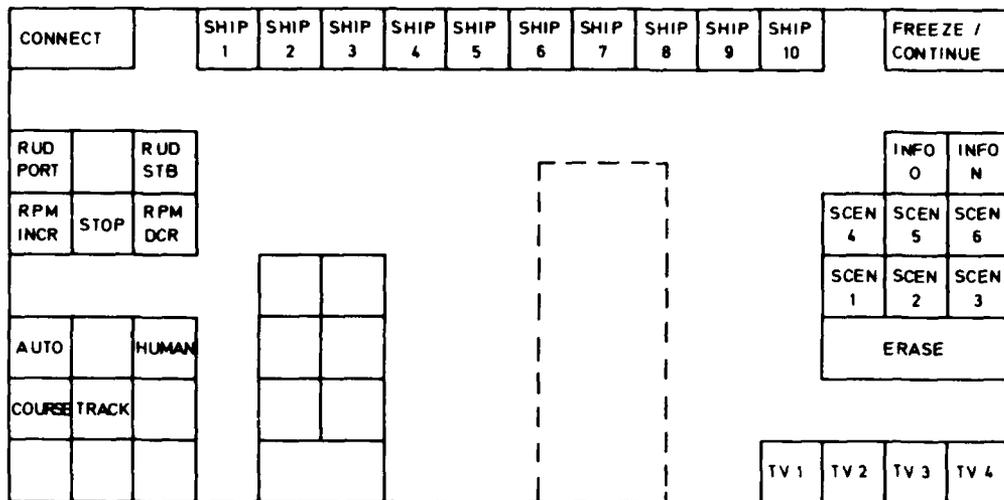
FIG. 4 Proposed Mansim Process console for "Instructor"
