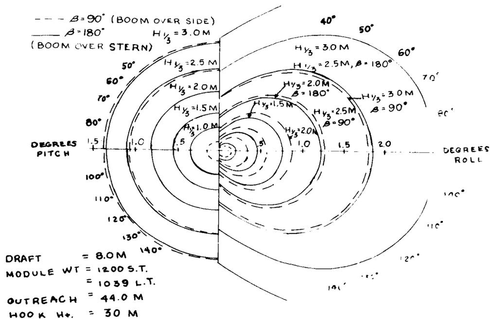
Figure 6. Onboard Guidance Chart.
