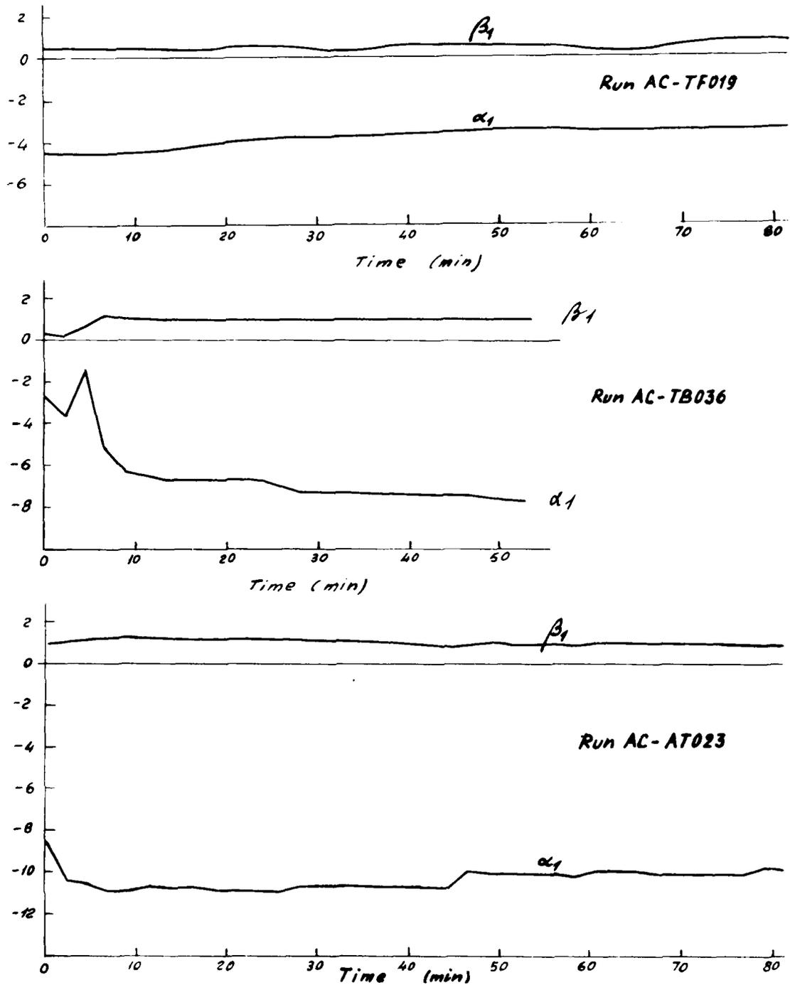
Figure 14: Model coefficients  $\alpha_1$  and  $\beta_1$  to show robustness of algorithm. Runs AC-TF 019 (tanker, full) AC - TB 036 (tanker, ballast) AC - AT 023 (containership).
