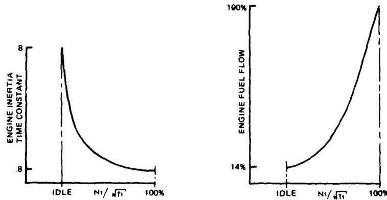
FIGURE 4 ENGINE STEADY STATE AND DYNAMIC CHARACTERISTICS
