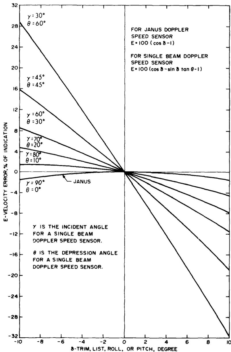
Figure 3. Velocity Error for Single Beam and Janus (Dual Beam) Doppler Sensors
