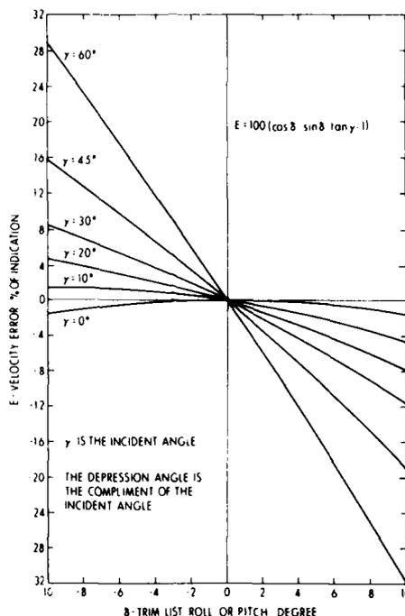
Figure 10. Correlation Speed Sensor Errors Caused by List, Trim, Roll, and Pitch
