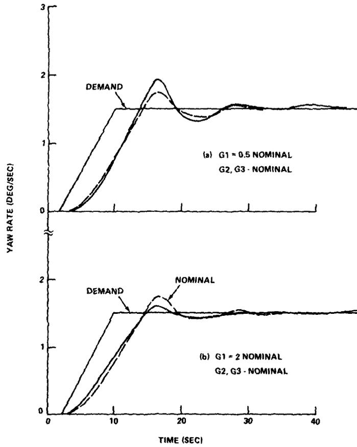
FIGURE 5. SENSITIVITY OF TURN RATE WITH RESPECT TO VARIATIONS IN G1 AT 40 kt
