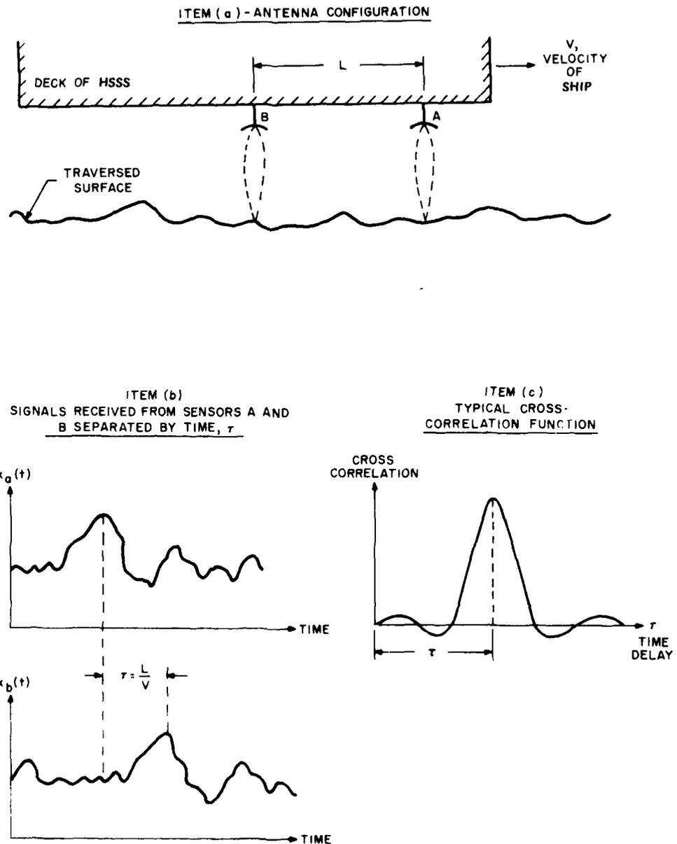
Figure 7. Cross-Correlation Speed Sensor
