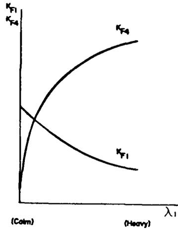
Fig. 3 Filter Gains vs.  $\lambda_1$  (Sea State)
