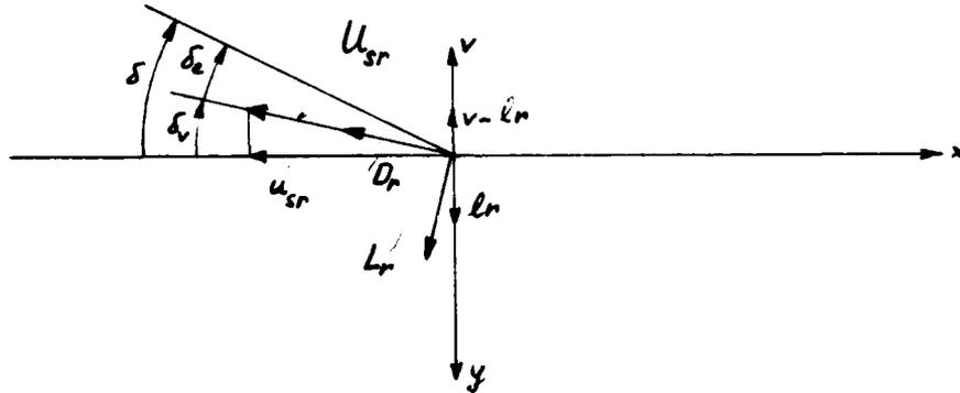
Figure 18: Relative speeds with respect to the rudder and forces on the rudder.
