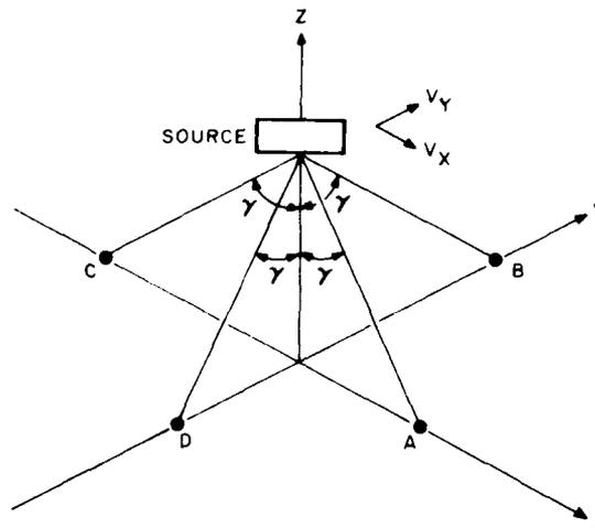
Figure 2. Geometry of a Janus Doppler System
