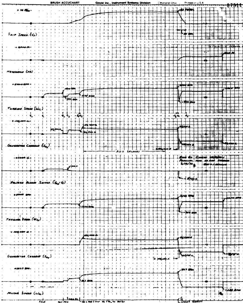
Figure 3. Standard Run: Two 15 MW Turbo-generator Systems
