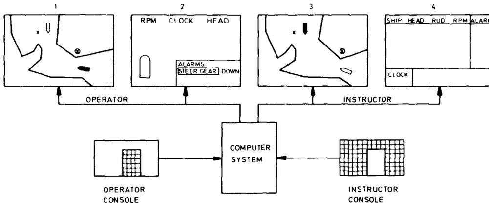
FIG. 7 Example of information on the four TV-screens in a collision study
