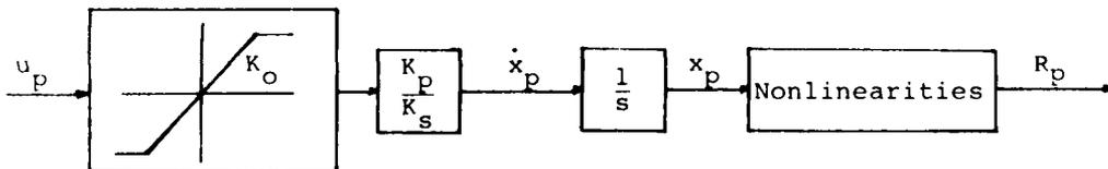
Figure 3. The Pitch Changing Mechanism.
