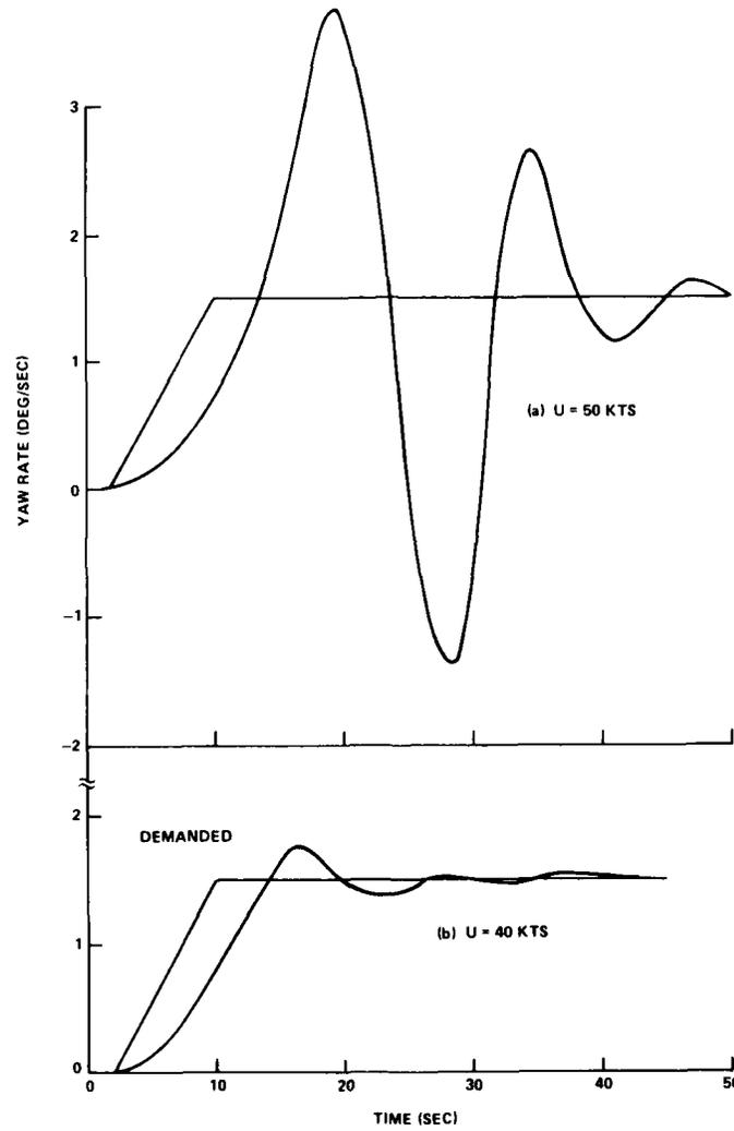
FIGURE 4. SIMULATED TURN RATES FOR JEFF(A) AUTOMATIC CONTROLLER TURNS AT 40 AND 50 kts WITH NOMINAL GAINS
