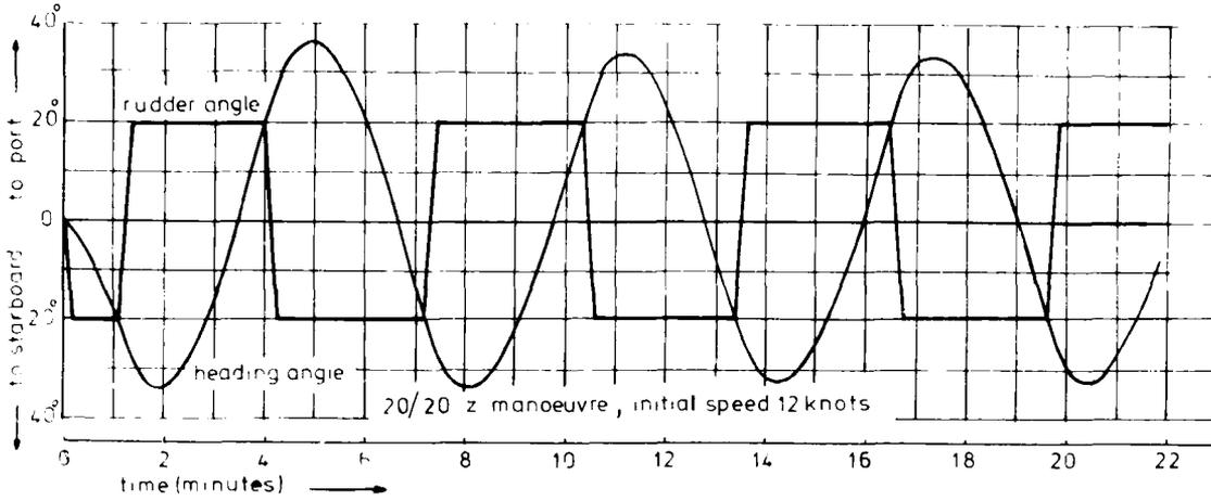
Figure 4: Second generation containership: zig-zag manoeuvre and turning circle.
