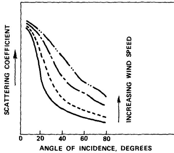
(a) Typical Scattering Coefficients for 1-3 cm Radar Over Water
