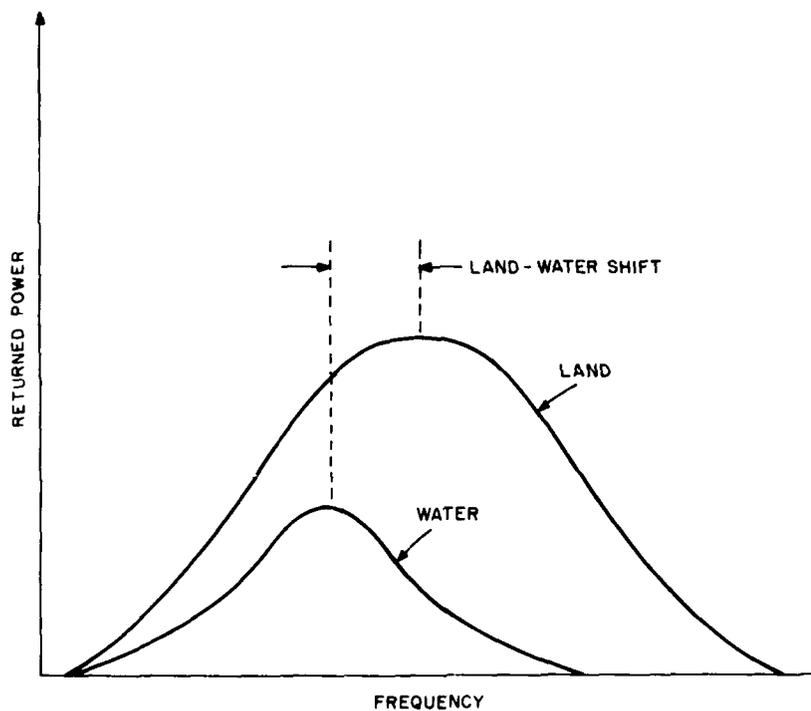
Figure 5. Doppler Frequency Spectrum for Land-Water Surfaces
