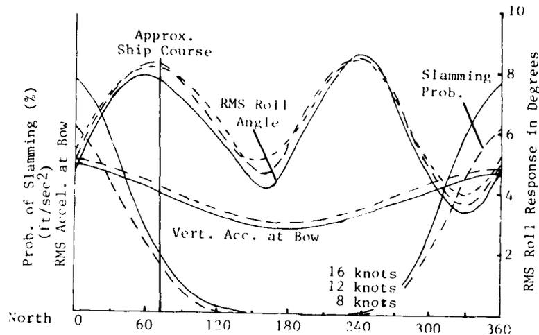
Figure 5. Variations of vertical acceleration at the bow, slamming probability and roll responses due to changes in heading and speed.
