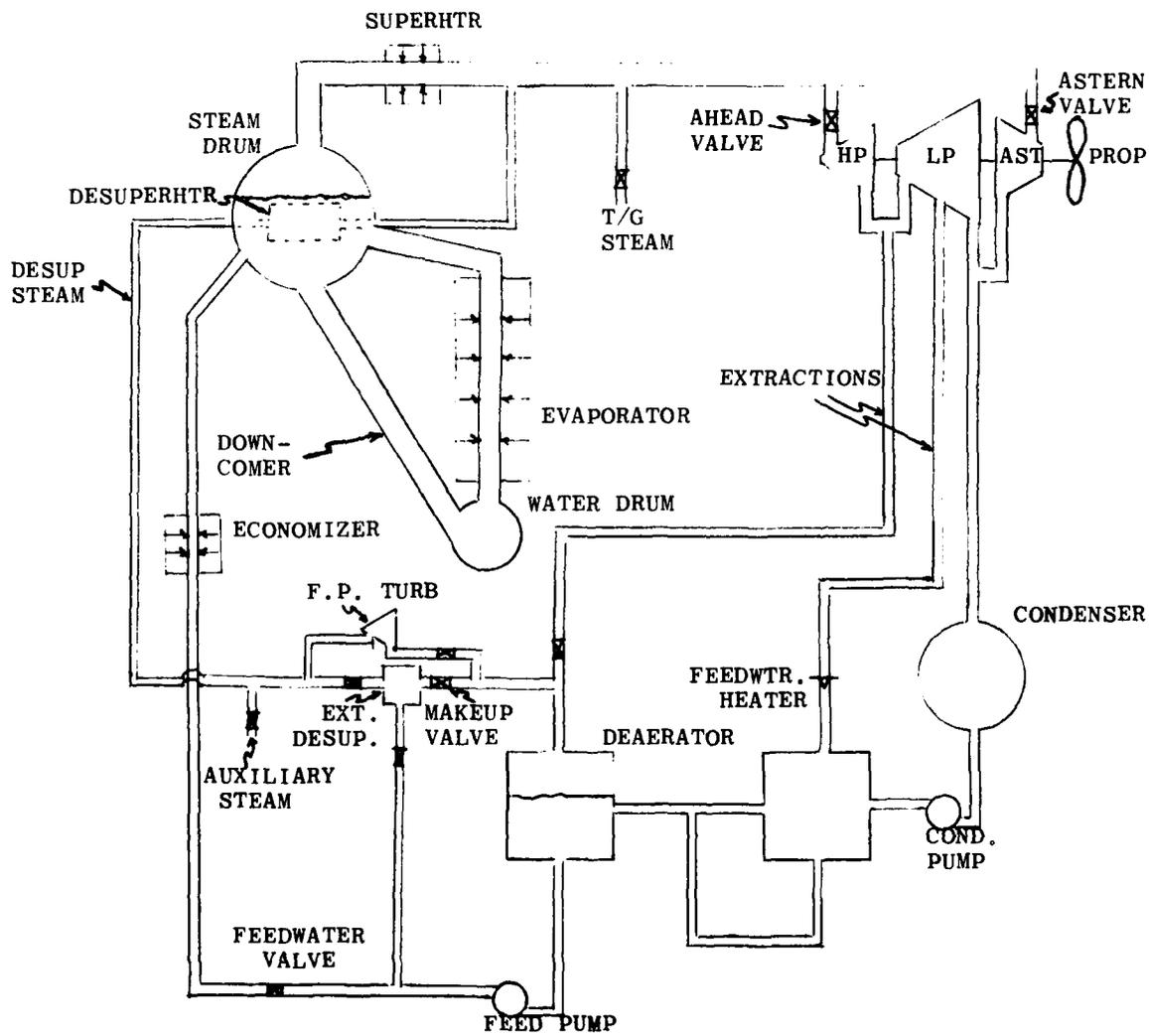
Figure 6. Block Diagram of Boiler Model
