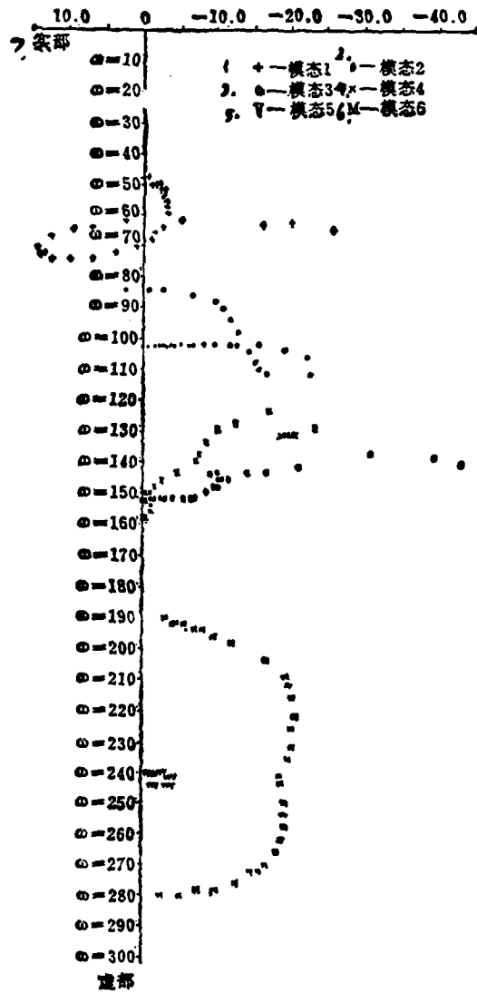
Figure 4. Root Locus Curves for the parabolic identification method of modes
