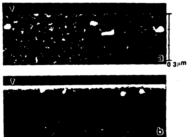
Fig. 3: XTEM weak-beam micrographs showing damage distributions in (a) direct RTA and (b) 550°C furnace plus RTA samples. Note dislocation loops in (b) are closer to the surface than (a). Arrow points to the sample surface.
