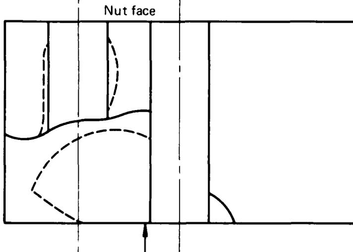
FIG. 6(c) FRACTURE SURFACES: SPECIMEN TYPE (D)
