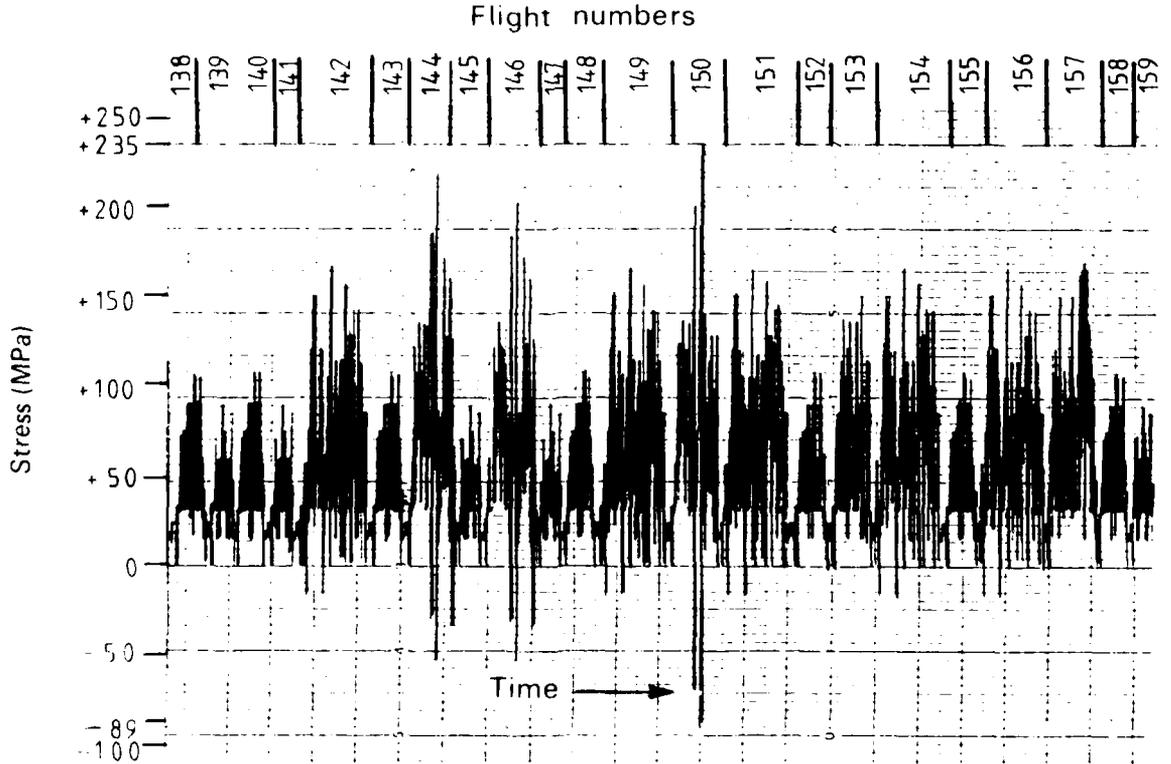
FIG. 5 STRESS SEQUENCE UNDER SWISS SPECTRUM ADJACENT TO FLIGHTS WITH  $+7.5g$  LOADS. ( $+7.5g = 235 \text{ MPa}$ )
