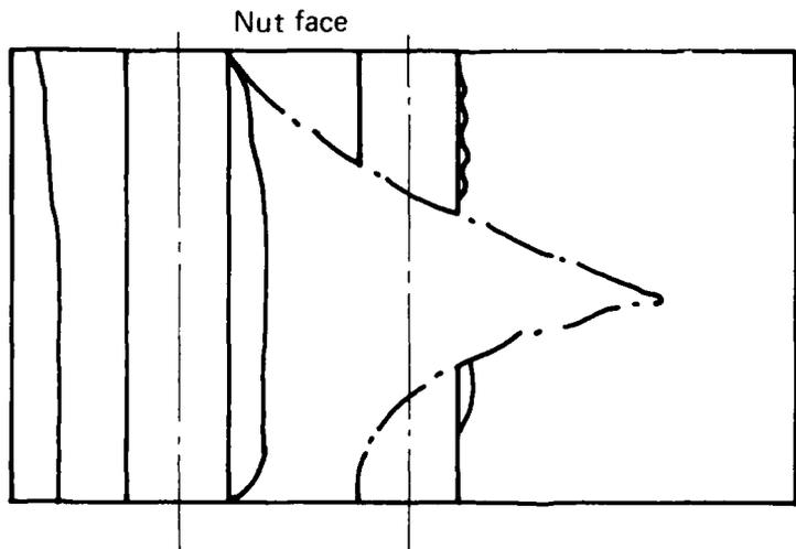
FIG. 6(b) FRACTURE SURFACES: SPECIMENS TYPE (C)
