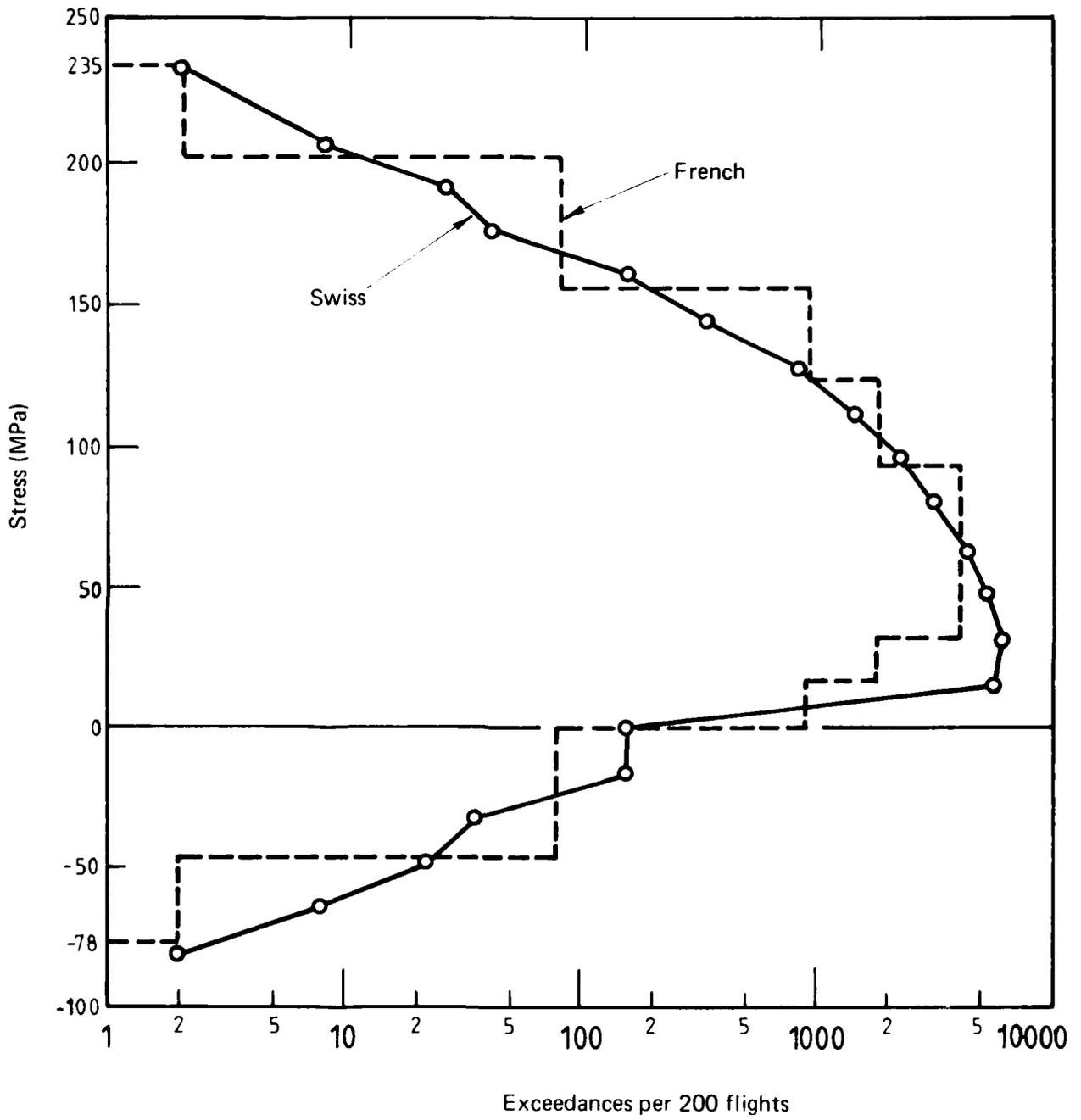
FIG. 4 STRESS SPECTRA FOR SWISS AND FRENCH SEQUENCES
