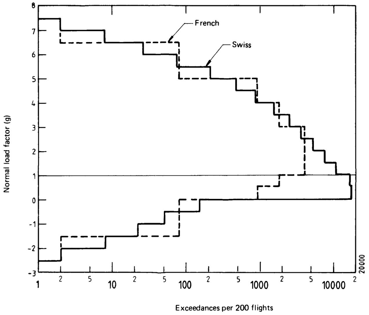
FIG. 1 LOAD SPECTRA FOR SWISS AND FRENCH TEST SEQUENCES
