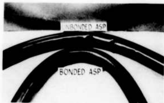
FIG. 3 COMPARATIVE BENDING OF ASP SHEATHS
