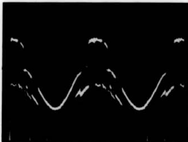
Fig. 1: Distorted, sinusoidal signal after having been transmitted via a single-mode fiber transmission system.
