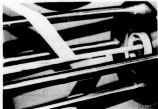
Fig. 16: Paper Tape Lapping of Cable on the Drum Twister
