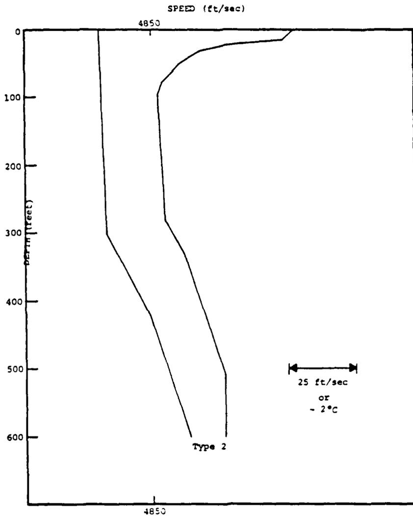
FIG.2.9 SOUND SPEED PROFILE (ENVELOPE TYPE 2) [REF.10]
