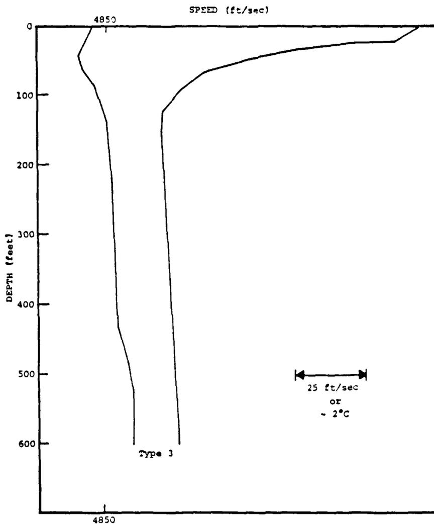
FIG.2.10 SOUND SPEED PROFILE (ENVELOPE TYPE 3) [REF.10]
