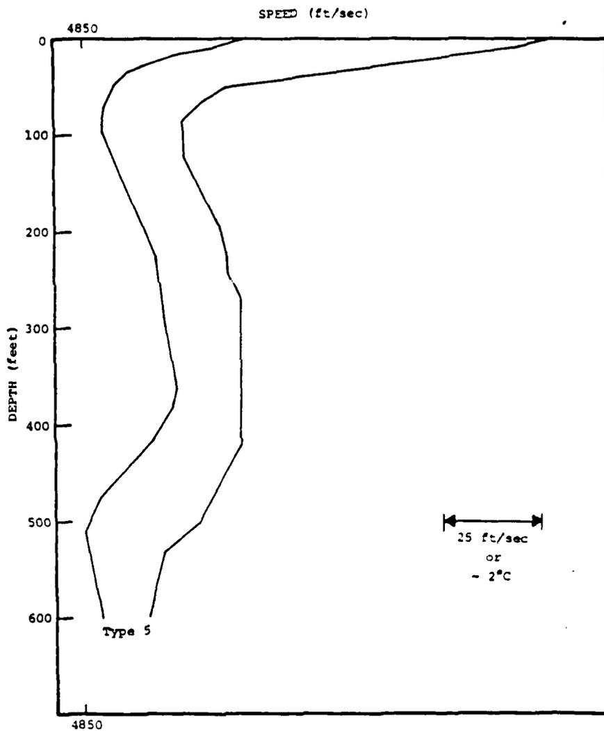
FIG.2.12 SOUND SPEED PROFILE (ENVELOPE TYPE 5) [REF.10]
