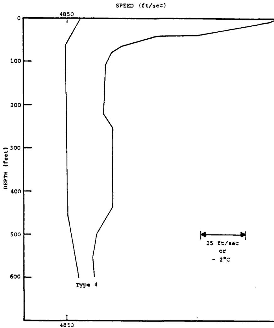
FIG.2.11 SOUND SPEED PROFILE (ENVELOPE TYPE 4) [REF.10]
