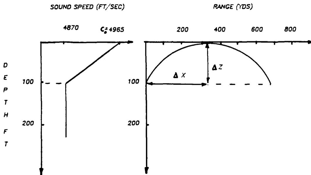
FIG.2.13 SURFACE REFRACTED RAY PATH
