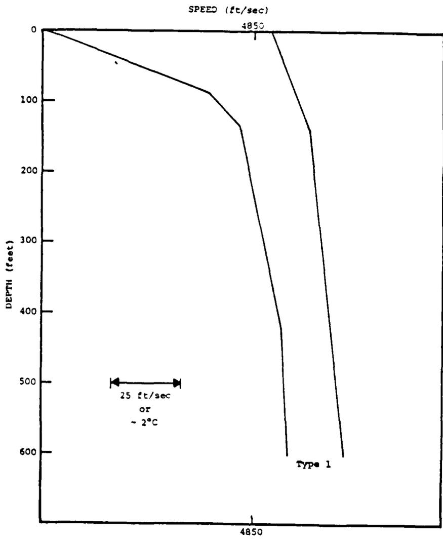
FIG. 2.8 SOUND SPEED PROFILE (ENVELOPE TYPE 1) [REF. 10]
