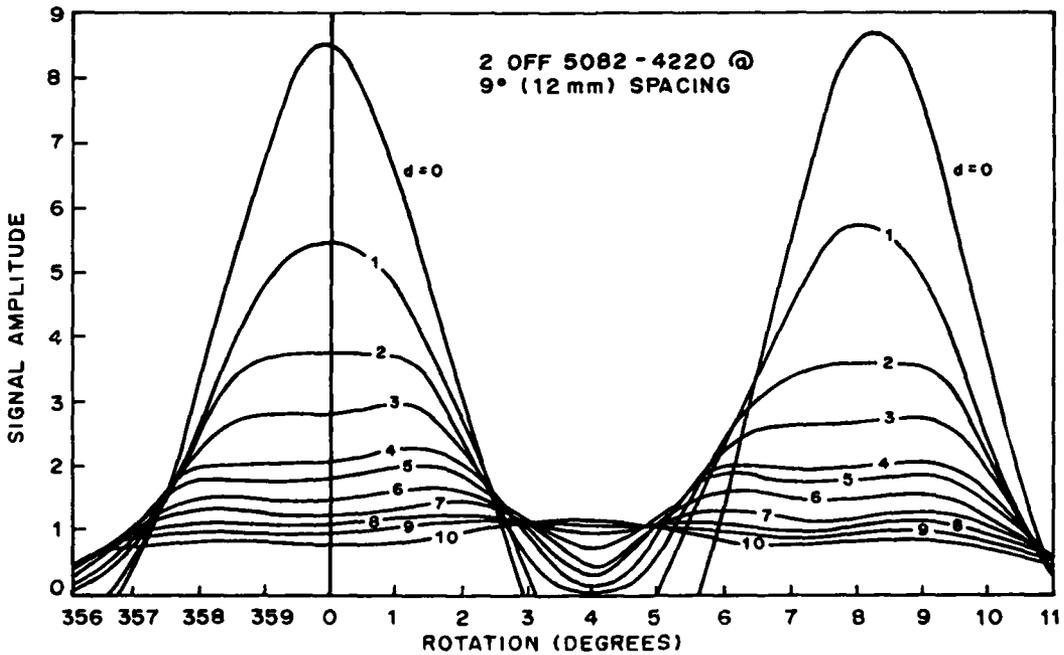
Figure 2. Effect of increasing separation between one IRED and two photodiodes
