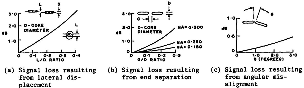
Figure 6. Light losses due to alignment problems
