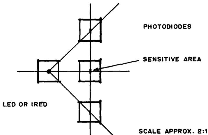
Figure 1. Simplified LED to photodiode relationship
