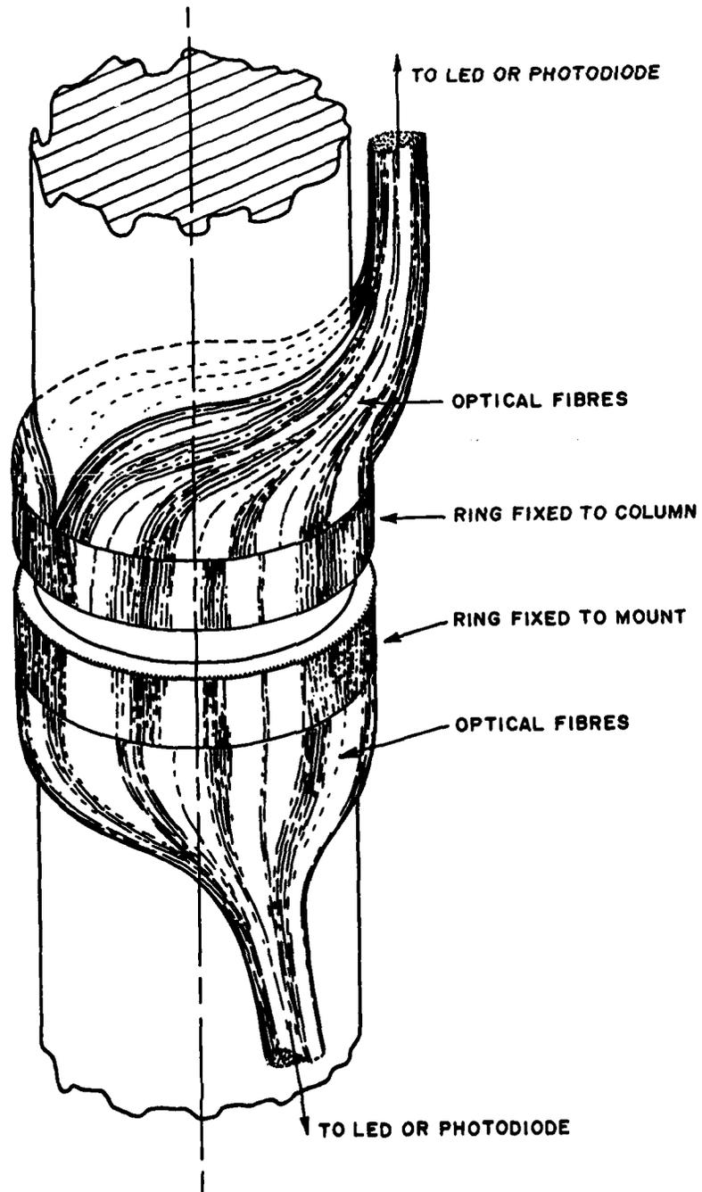
Figure 5. "Ring of Fibres" slip-rings
