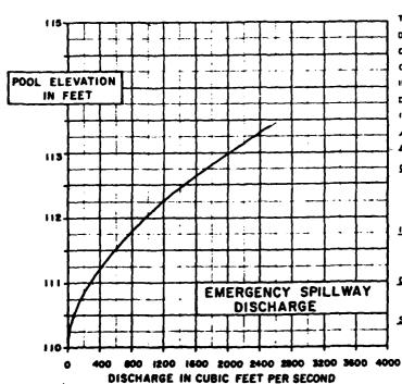
TOP OF DAM EL 116.0 EL 112.4 DESIGN HIGH WATER CREST EMERGENCY SPILLWAY EL. 110.0 CREST PRINCIPAL SPILLWAY EL. 100.0 DRAINAGE AREA CONTROLLED 1.90 SO MI. I" OF RUNOFF = 101.33 ACRE-FEET ALL ELEVATIONS REFER TO METROPOLITAN DISTRICT DATUM
