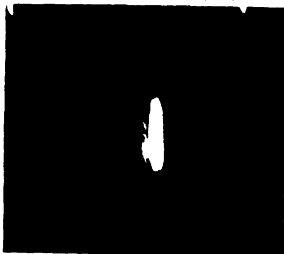
Figure VI-10. Far-field of output prism-coupled waveguide. Fabricated by ion-exchange in a superlattice sample of \text{GaAs}/\text{AlGaAs} of 100\text{ nm} period. A 100\text{ nm} wide waveguide was etched into the surface. The waveguide was coupled to a 100\text{ nm} wide output waveguide.
