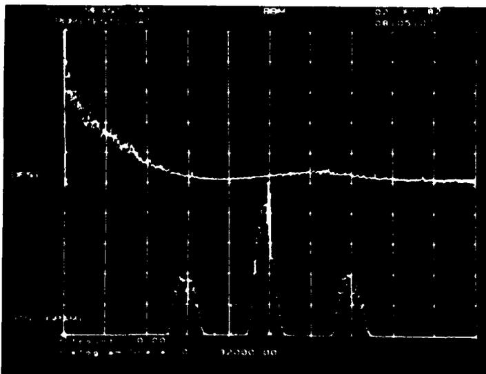
count. In this case the count is zero, but lines showing the edges of the hit region appear anyway. The DFS here is typical of the no-interference Vicom T1-4000.
