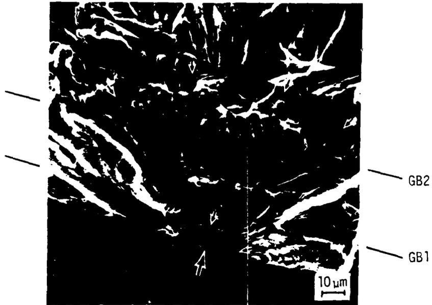
Fig. 4: a) Micrograph showing the changes in the direction of crack advance when the crack tip encounters a grain boundary.
