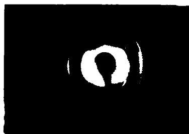
Figure 1. X-ray diffraction pattern of oriented \gamma -phase PVF 2 .
