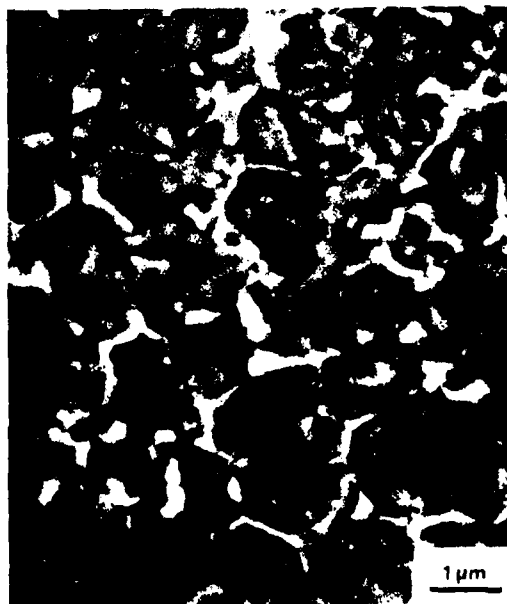
Figure 7. As-atomized powder, <37 μm; Kalling's etch. SEM.
