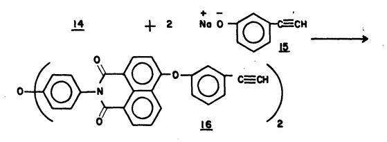
Differential Scanning Calorimetry (DSC) analysis showed <u>16</u> to be crystalline and have a doublet melting point at 211° and 216°. These were followed by a doublet exotherms at 249° and 261° corresponding to the onset of polymerization. In addition the diacetylene <u>16</u> could be fabricated into films suitable for hydrolysis studies.
