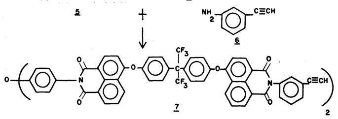
The DSC Thermogram of  $\underline{7}$  showed a glass transition temperature of 226° with a polymerization onset temperature of 240°C. The proximity of the two temperatures made fabrication impossible.
