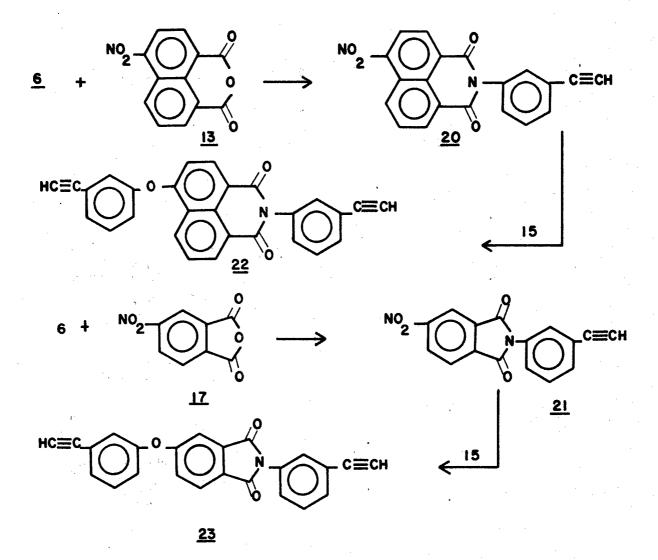
The imide 22 by DSC analysis exhibited a melting point of 205°C and 133°C for 23. When the resins were heated through the melting point to the beginning of the polymerization exotherm and then cooled slowly, all crystallinity was lost and a Tg of 78°C for 22 and 3°C for 23 resulted.
