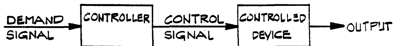
FIGURE 3-1 BLOCK DIAGRAM - OPEN-LOOP CONTROL MODE
