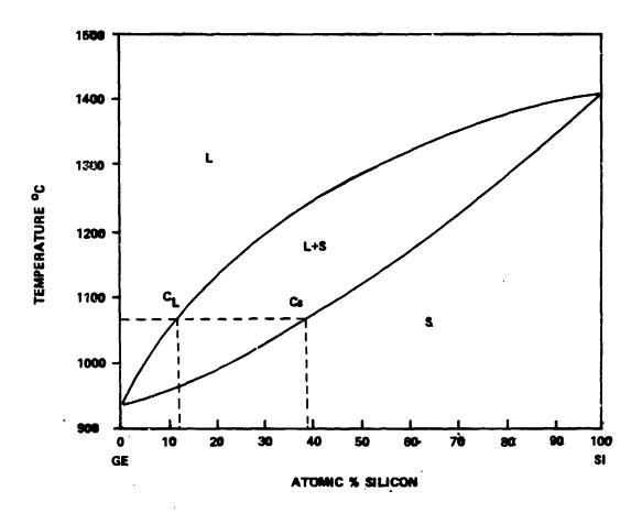
Figure 4. Germanium-Silicon Phase Diagram.
