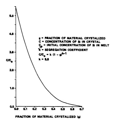
Figure 6. Concentration Profile of Silicon in Germanium.
