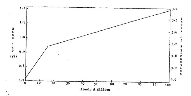
Figure 1. Band Gap and Refractive Index vs. Alloy Composition.
