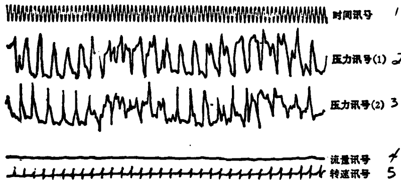
Fig.8 The oscillograms measured by two pressure transducers in transient process of rotating stall at n=13000\text{rpm} (transducers located at the tip of the blade)
