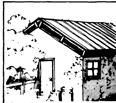
Provide man-made shade for the building by using a double roof with an open space between.
