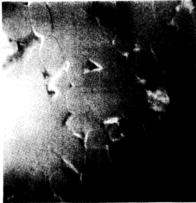
Figure 3 SEM photomicrograph of sample SN502-95-12 which was fired at 2145^{\circ}\text{C} under 2.2 MPa of \text{N}_2 for 30 minutes. (10,000 X).
