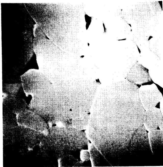
Figure 5 SEM photomicrograph of sample SN502-95-14 which was fired at 2145°C under 2.2 MPa of N 2 for 30 minutes in the 1st step and 2045°C under 2.2 MPa of N 2 for 30 minutes in the 2nd step. (10,000 X).
