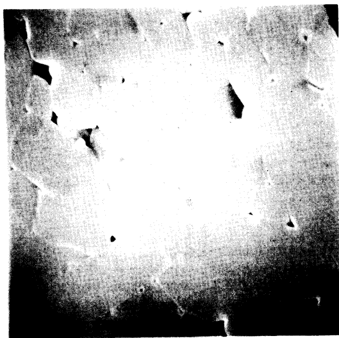
Figure 6 SEM photomicrograph of sample SN502-95-15 which was fired at 2145°C under 2.2 MPa of N 2 for 30 minutes in the 1st step and 2045°C under 2.2 MPa for 30 minutes in the 2nd step. (10,000 X).
