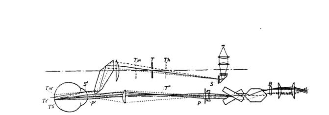
Figure 3. The essential optics in Fincham's (1937b) coincidence optometer.
