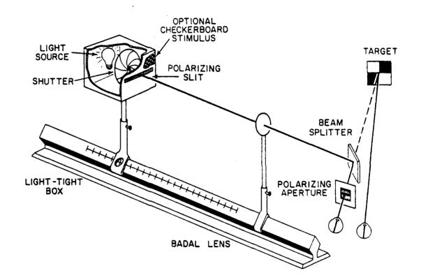
Figure 9. Scnematic of polarized vernier optometer (not shown is the diffusing glass placed between the lamp and shutter to eliminate "hot spots" in the vernier).
