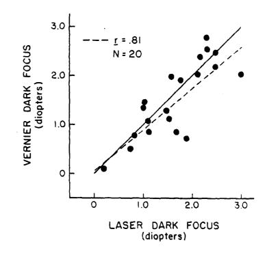
Figure 11. Agreement of dark focus readings taken with the laser and vernier optometers.
