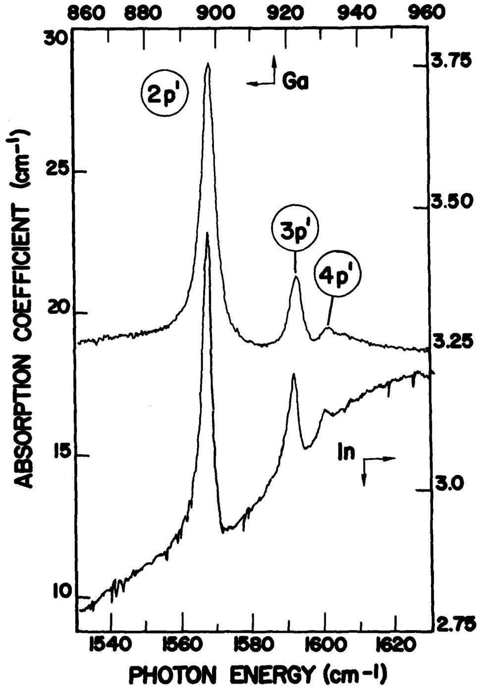
Figure 3. Absorption Spectra ( $p_{1/2}$  Series) for Gallium and Indium in Silicon. Gallium Concentration and Sample Thickness Same as for Figure 1. Indium Concentration  $4.2 \times 10^{16} \text{ cm}^{-3}$ . Indium Sample Thickness 0.397 cm. Resolution =  $0.5 \text{ cm}^{-1}$ .
