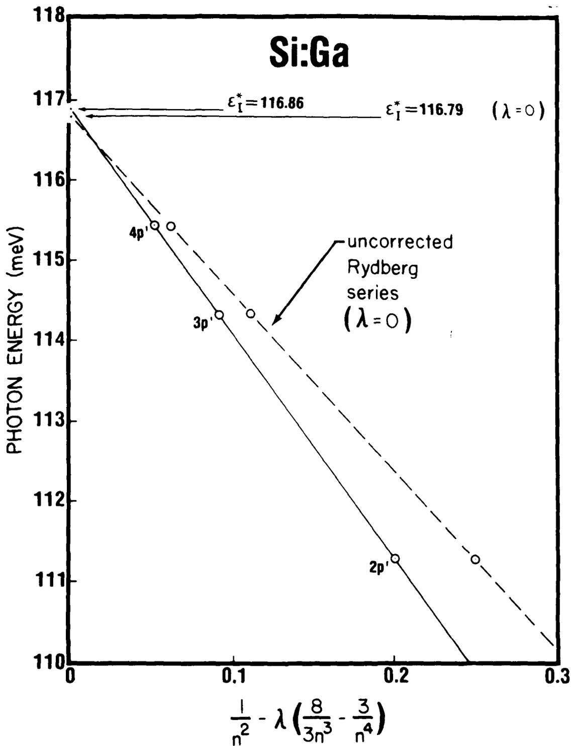
Figure 4. Plot of Uncorrected Rydberg Series (Dashed Line) and Corrected Rydberg Series (Solid Line) for  $p_{1/2}$  Lines of Gallium in Silicon.
