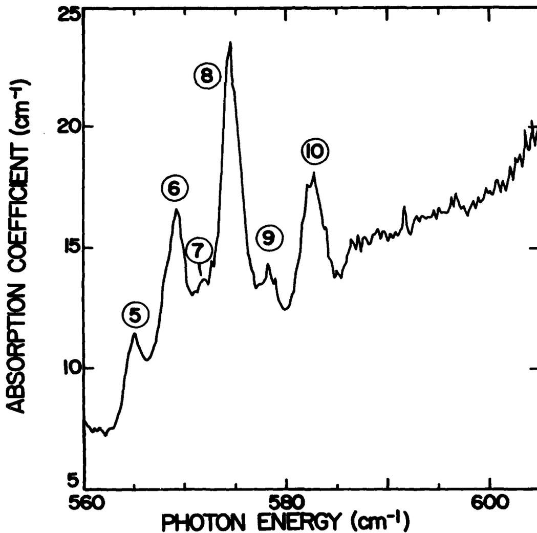
Figure 2. Expanded Absorption Spectrum for Gallium in Silicon in the Region Containing Lines 5 through 10 of the  $p_{3/2}$  Series. Sample Thickness 0.175 cm. Resolution =  $0.5 \text{ cm}^{-1}$ .
