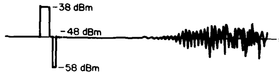
Figure 9b. Power Received From 75 m Cable From a Monopole 15 m Above Ground
