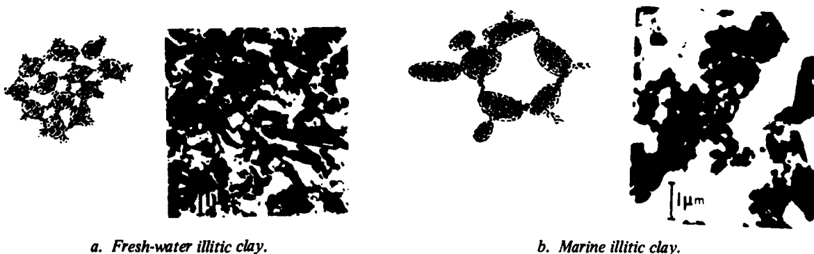
Figure 123. Clay microstructure as observed in a transmission electron microscope using ultrathin acrylate-treated specimens. Left pictures show schematic, generalized patterns; dark parts represent mineral substance (from Andersland and Anderson 1978).
