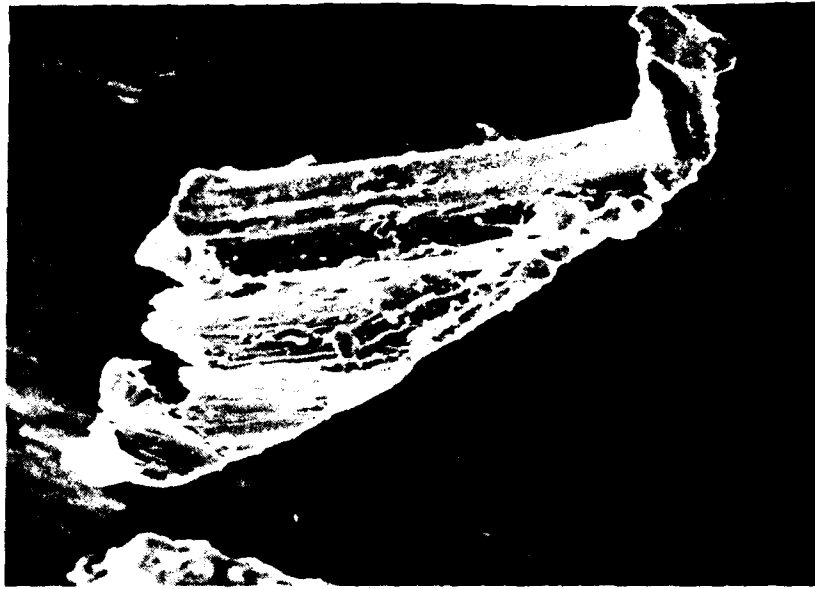
A. Erosion Debris Particle (Magnification: 660X)
