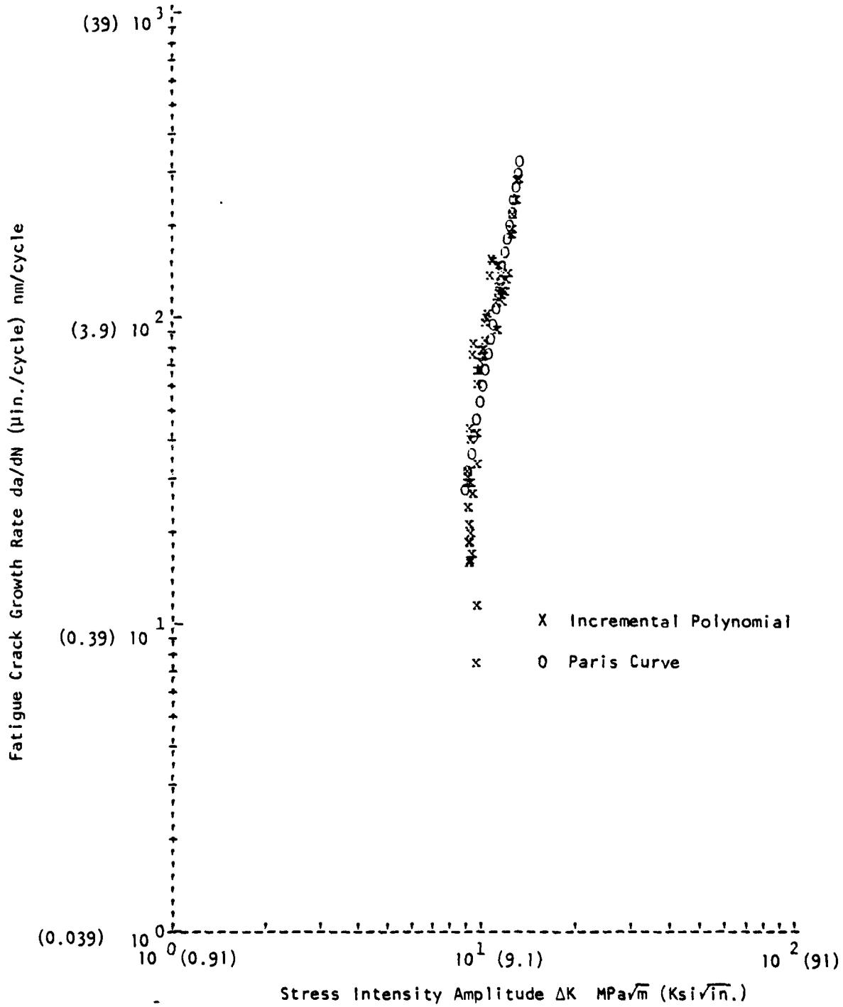
Figure A-1b. Paris Curve Fit, TL Orientation
