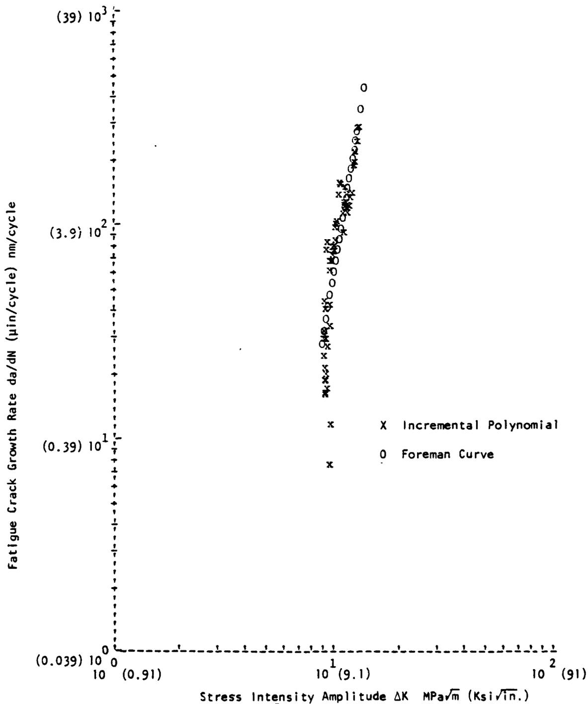
Figure A-2b. Foreman Curve Fit, TL Orientation
