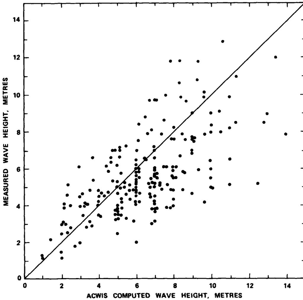
Figure 6. Measured  $H_s$  versus computed  $H_s$  cross plot for paired data<sup>s</sup> (excluding NDBO buoy<sup>s</sup> data)
