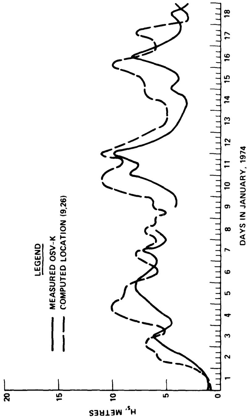
Figure A7. Comparison plot of  $H_s$  versus time for a period in January 1974 at OSV-K
