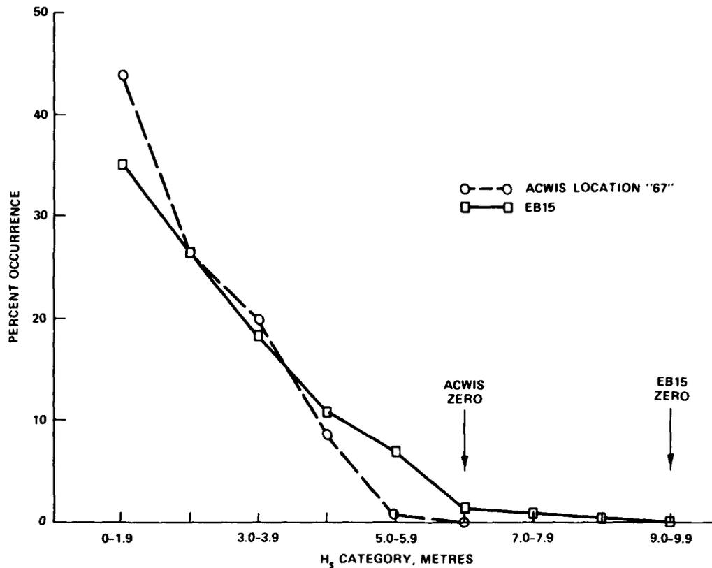
Figure 4. Plot of percent occurrence versus  $H_s$  for measured (buoy) data and computed data. Notice the ACWIS computed no waves over 6 m (ACWIS zero); yet EB15 recorded some waves above 8 m
