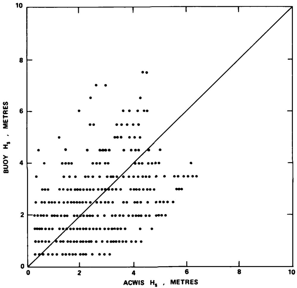
Figure 7. Measured  $H_s$  versus computed  $H_s$  cross plot for paired NDBO buoy data
