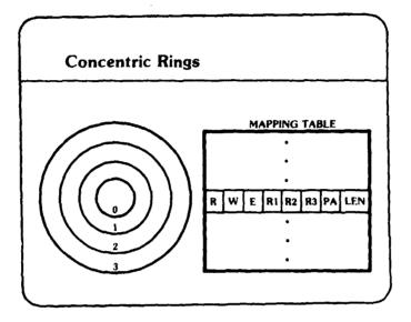
Concentric ring hardware architectures are a generalization of hierarchical execution domain architectures. The MULTICS 6180, Honeywell SCOMP, and PRIME 400 and 500 are examples of concentric ring architectures. This slide illustrates the general characteristics of a ring architecture supporting a segmented virtual memory.
