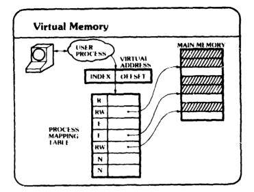
Here is a rather generalized description of virtual memory. It is meant to characterize both true virtual memory systems, such as MULTICS and VAX-11/780, and so-called mapped memory systems like the PDP-11/45 and 11/70.
