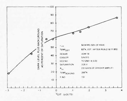
Fig. 16. Dark level plus background vs.  $V_{\mbox{G1T}}$  at 50% integration.
