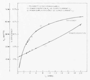
Fig. 10. Power dissipation vs. output current ( $I_0$ ) of Abbott Transistor Labs Model CC15D1.0 power supply ( $^{\pm}15-V$ , 1.0 A each output).
