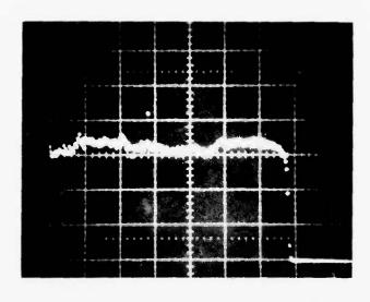
A. OUTPUT OF ARRAY AT 25% INTEGRATION (27.32 ms)
