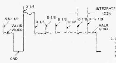
B. ILLUSTRATION OF VALID VIDEO TRANSFER AT 12.5% INTEGRATION (X-fer 1/8) AND ASSOCIATED 1/4 AND 1/8 INTEGRATION DUMPS (D 1/4 AND D 1/8)
