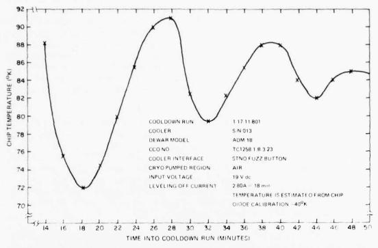
Fig. 26. Variation of chip temperature with cooldown time (run 1-17-11-801).
