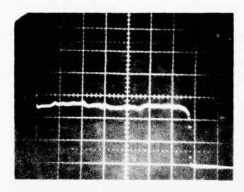
A, OUTPUT OF ARRAY AT 12.5% INTEGRATION (13.66 ms)
