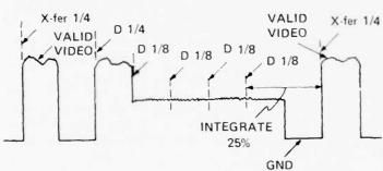
B. ILLUSTRATION OF VALID VIDEO TRANSFER AT 25 % INTEGRATION (X-fer 1/4) AND ASSOCIATED 1/4 AND 1/8 INTEGRATION DUMPS (D 1/4, D 1/8)
