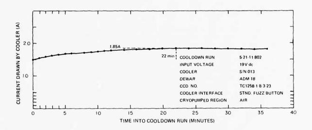
Fig. 32. Current drawn by cooler S/N 013 following use of the cooler in eight prior cooldown runs.
