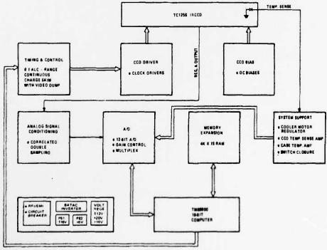
Fig. 2. Sensor Unit electronics block diagram (ADM-1).
