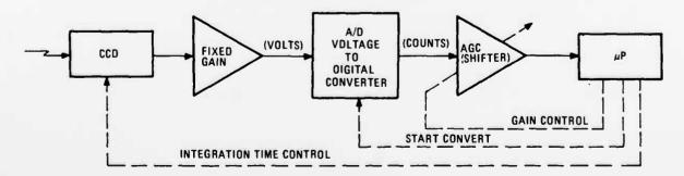
Fig. 40. System configuration with automatic level control.
