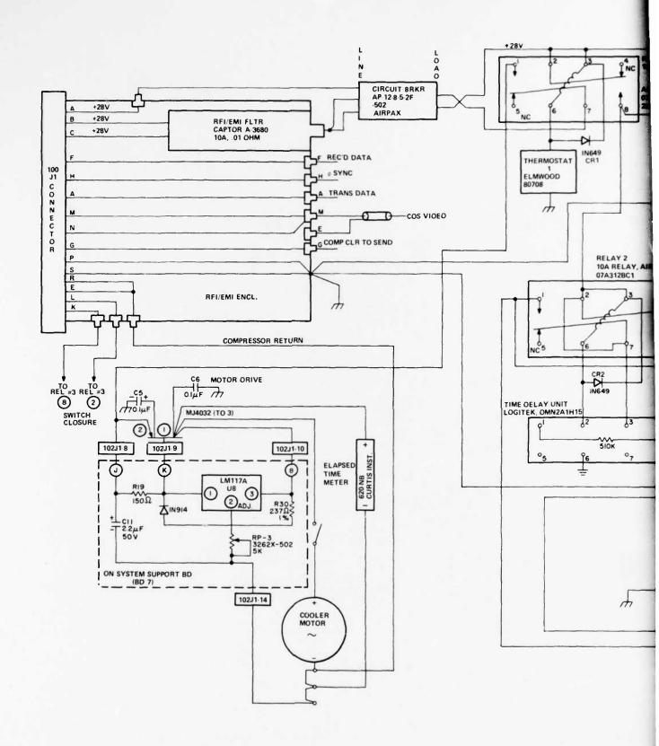
Fig. 3. Power conditioning and control circuitry.
