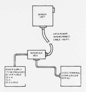
Fig. 1. Arrangement of the ADM-1 system major assemblies.
