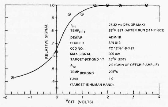
Fig. 17. Relative signal response vs.  $\rm V_{G1T}$  at 25% integration.
