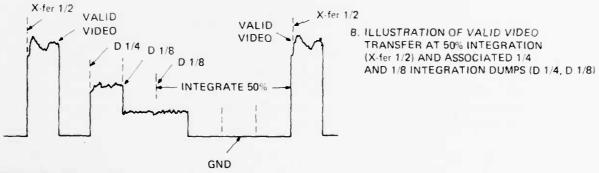
CCD NO. TC1258·1·8·3·23 DEWAR ADM-18 COOLER S/N 013 CHIP TEMP, =  $83^{\circ}$ K (EST) FOLLOWING RUN 2·18·11·802 SATURATION = 3.35 V (AT INPUT TO A/D) OFFCHIP VOLTAGE GAIN = 2.0 T<sub>BCKGND</sub> =  $295^{\circ}$ K (EST) F/NO = 1.0
