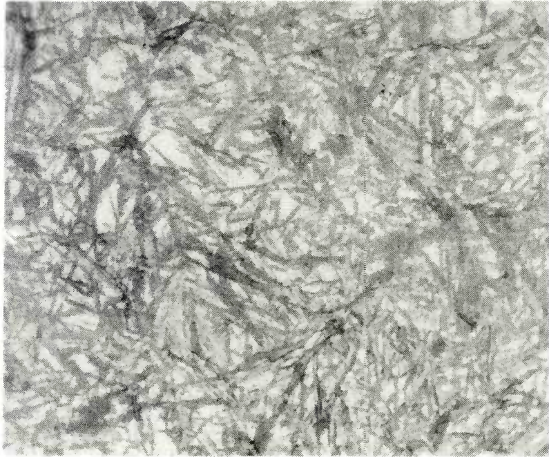
Figure 23. Photomicrograph of untempered martensite with some retained austenite (white area) in sample austenitized at 843°C (1550°F). 1000x
