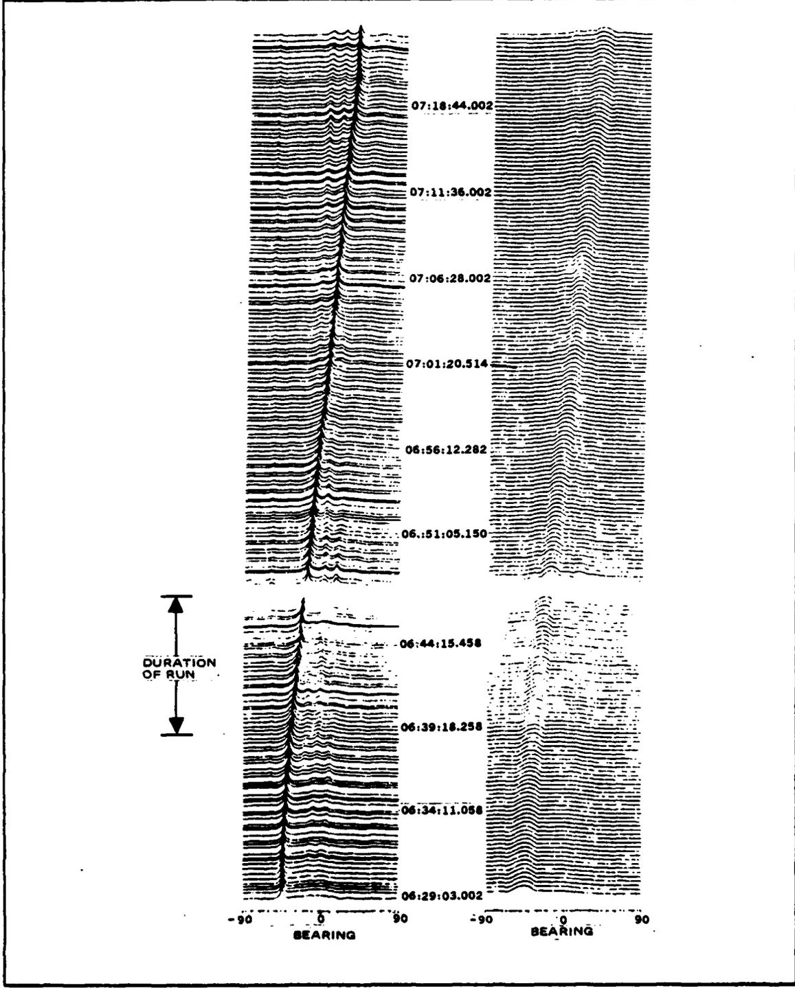
Figure 20. Bearing Time Plot for HOTEL-1 Exercise with Beamforming
