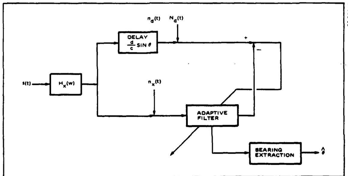
Figure 8. Equivalent Model for Split Array Tracker in Special Case
