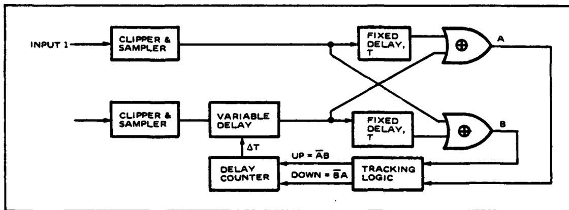
Figure 13. Two Point Correlator Tracker Block Diagram
