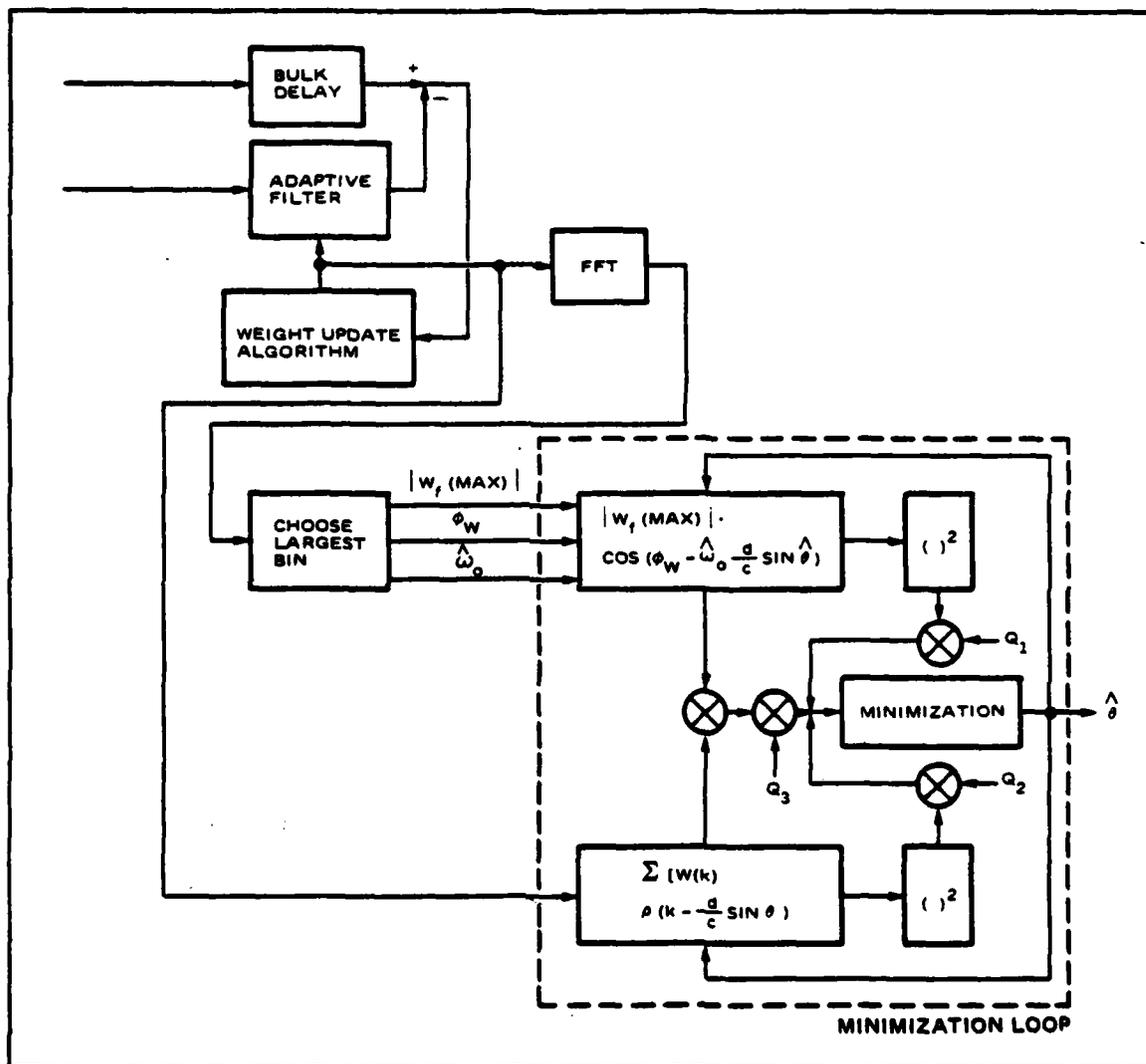
Figure D1. Combined Adaptive Tracking System with Unknown SNRs
