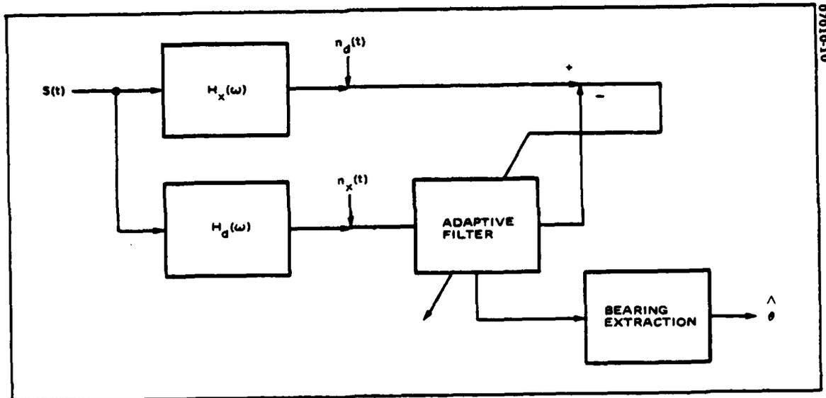
Figure 7. Equivalent Model for Split Array Tracker
