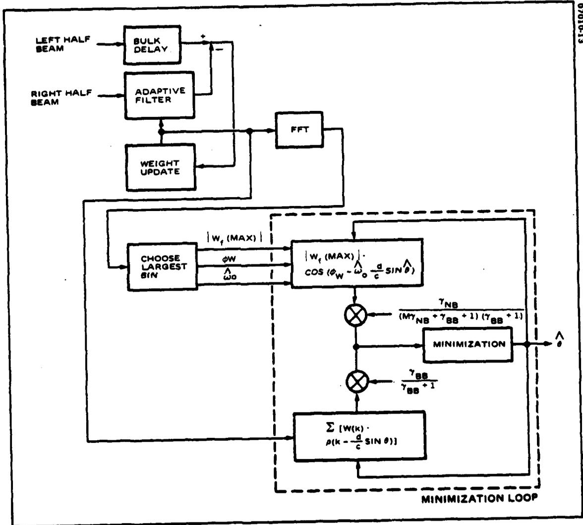
Figure D2. Combined Estimator with Known SNRs
