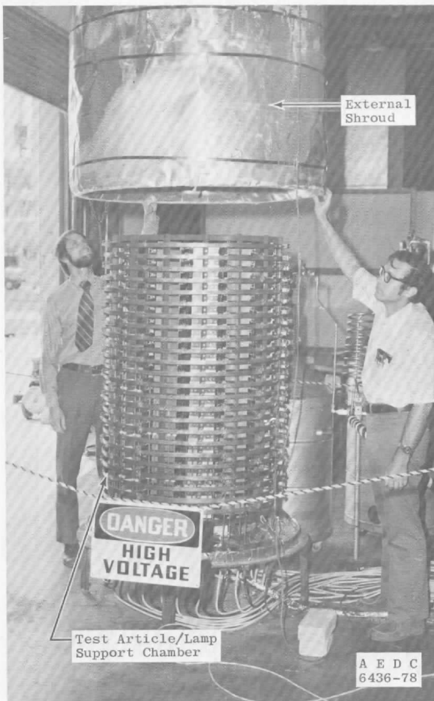
Figure 11. Radiant-heat test stand and external shroud.
