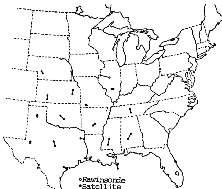
Fig. 24. Pairings of satellite sounding locations and rawinsonde stations at 2100 GMT on 10 April 1979.
