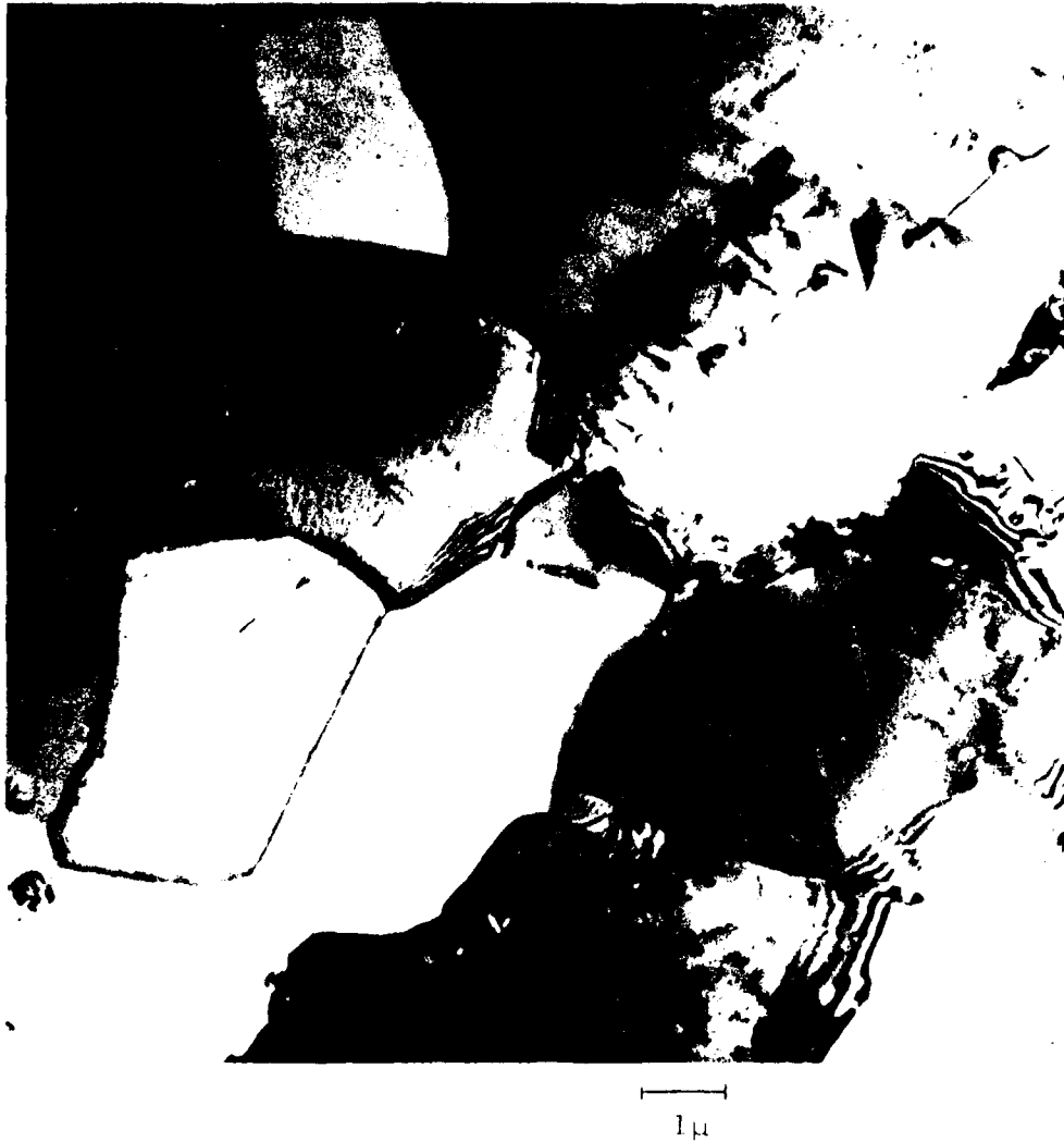
FIGURE 4-45. TEM OF Al-Li-Zr (#26A) SHEET Aged 400°F/50 minutes (underaged). 11,500X.
