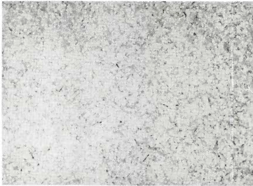
Figure 62. Photomicrograph Showing the Microstructure of the Subject Blades. Magnification: 500X; Etchant: Dilute Marbles
