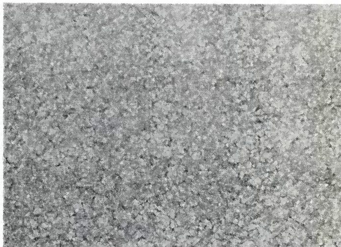
Figure 17. Orthogonal Sections Showing Microstructure of AM-350 Feedstock. After Annealing, Cold Draw/Roll Forming of Preform Equalizing and Overtempering. Etchant: Marble's (10 sec); Magnification: 500X
