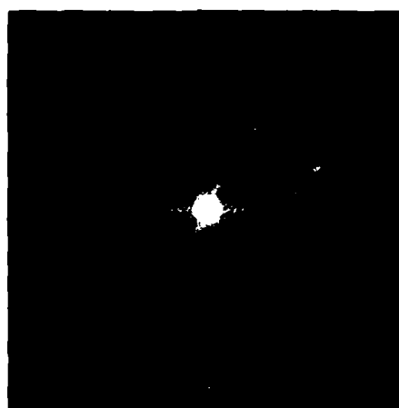
(b) Fourier transform of radar image of rural field region
